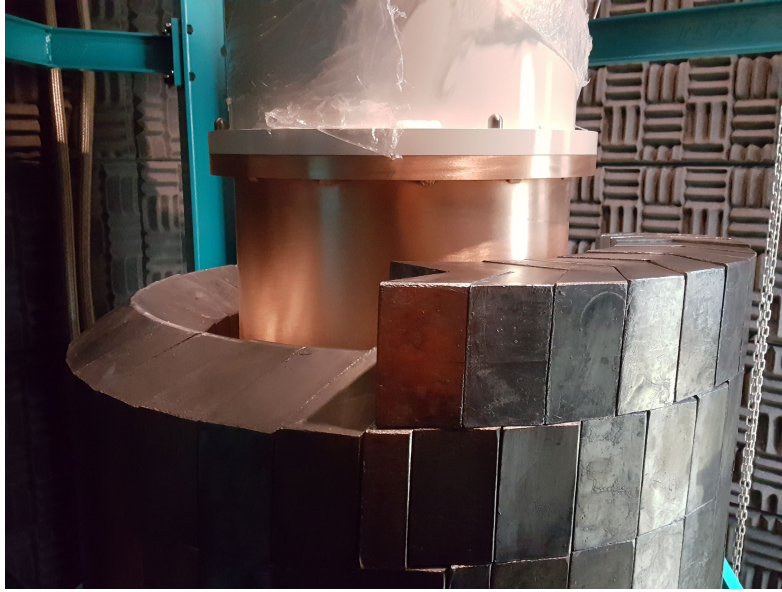
FIGURE 2.12: View of the CROSS cryostat and a 15 cm layer of lead shielding.
