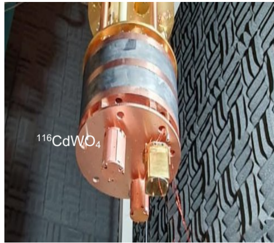
FIGURE 5.7: ^{116}\text{CdWO}_4 scintillating bolometer fixed on the 10 mK plate of the C2U cryostat.
