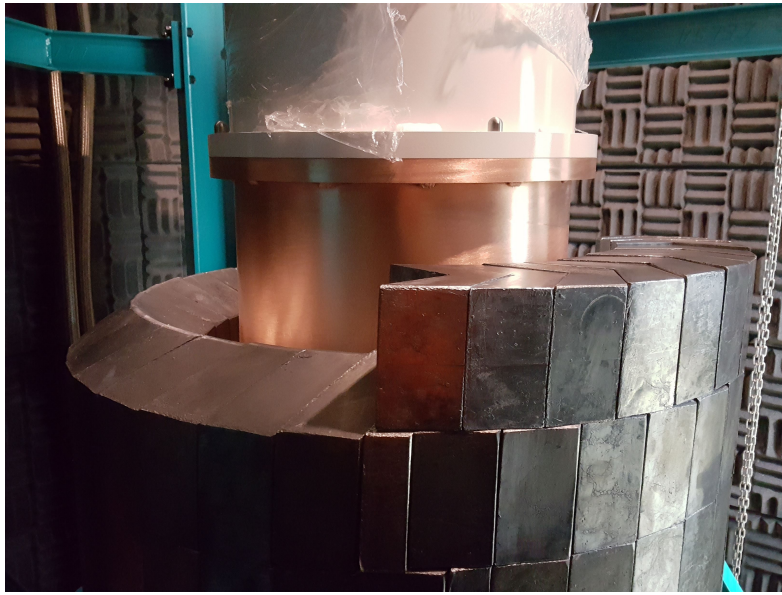
FIGURE 2.12: View of the CROSS cryostat and a 15 cm layer of lead shielding.
