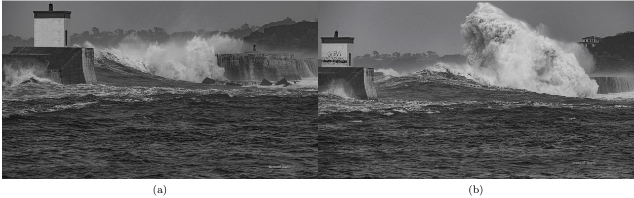
Figure 3.26: Photographs of a wave impact during a storm event at the sensor location on December 9 2019 around 4pm. H_s = 5.9m , T_p = 15s , wl = 2.9m , courtesy of Bernard Bayle
