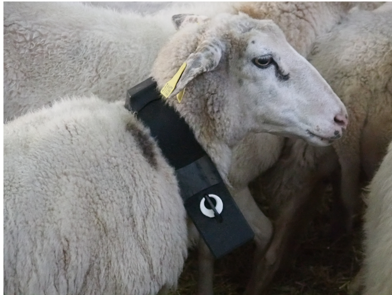
Figure 4.1 – An accelerometer mounted on a sheep’s collar.
