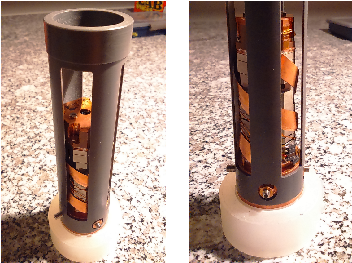
Figure A.3: Sample ready to be installed in the vacuum chamber of the cryostat. The piezomotors and the thermistor are electrically connected, a double propeller of copper foils is realized in order to establish a thermal transfer to the sample. The piezomotors are mounted on a translation micrometer stage which is itself fixed to an insulating plastic tube providing support to the assembly. To achieve good thermal transfer of the sample, the copper foils must under no circumstances be in contact with the plastic tube.
