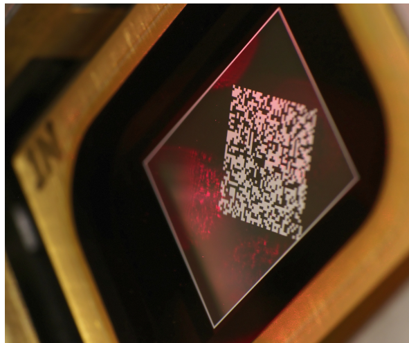
Figure 2.9: Image of a random 31 \times 31 matrix \mathbf{W}^{\text{DMD}} on the digital micro-mirrors device. Each white or black pixel is an array of 18 \times 18 DMD pixels. Only the white super-pixels are turned towards the output detector.
