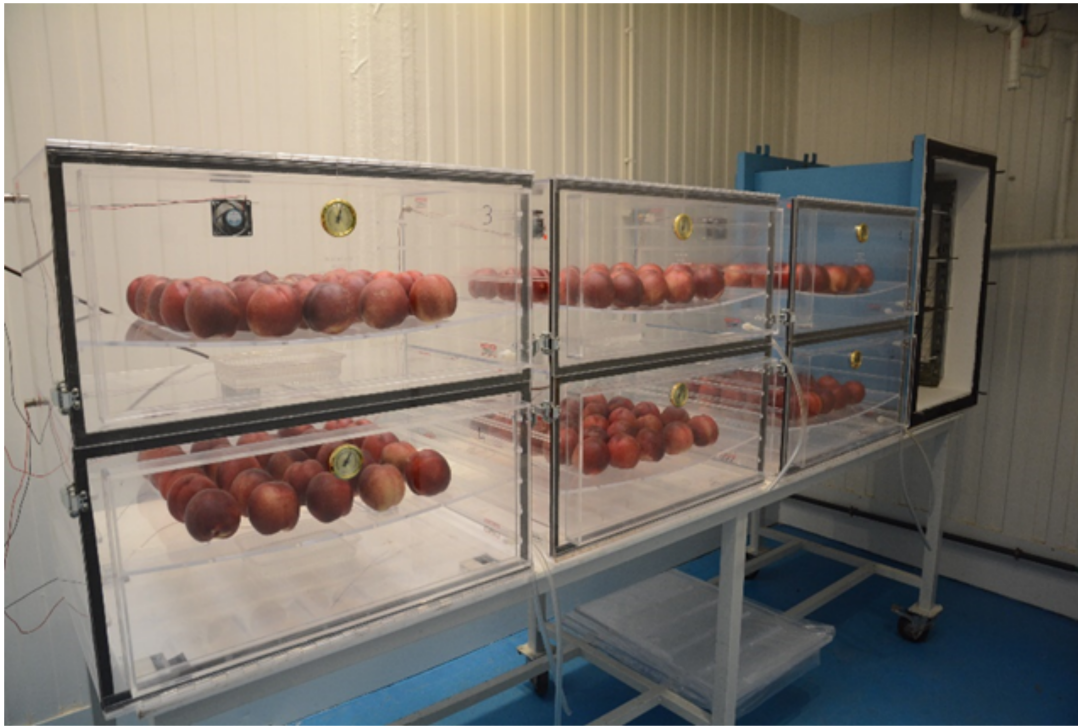
Figure 2.1 – Experimental set-up for the brown rot secondary infections experiment. The three upper cells contain a central inoculated fruit (I), while the lower are the control groups (C).
