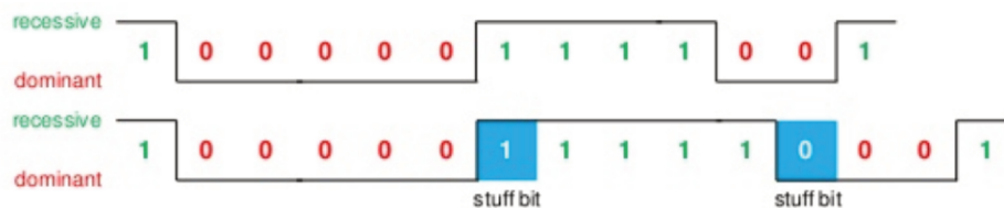
Figure 2.6: Bit stuffing example mbedlabs (2016)
