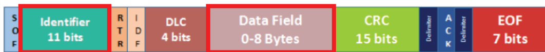
Figure 5.1: CAN message frame, We highlight the fields used to create the dataset. The ID defines the content, and Payload is the Encoded Signals. Each message is timestamped whenever the transmission is captured.
