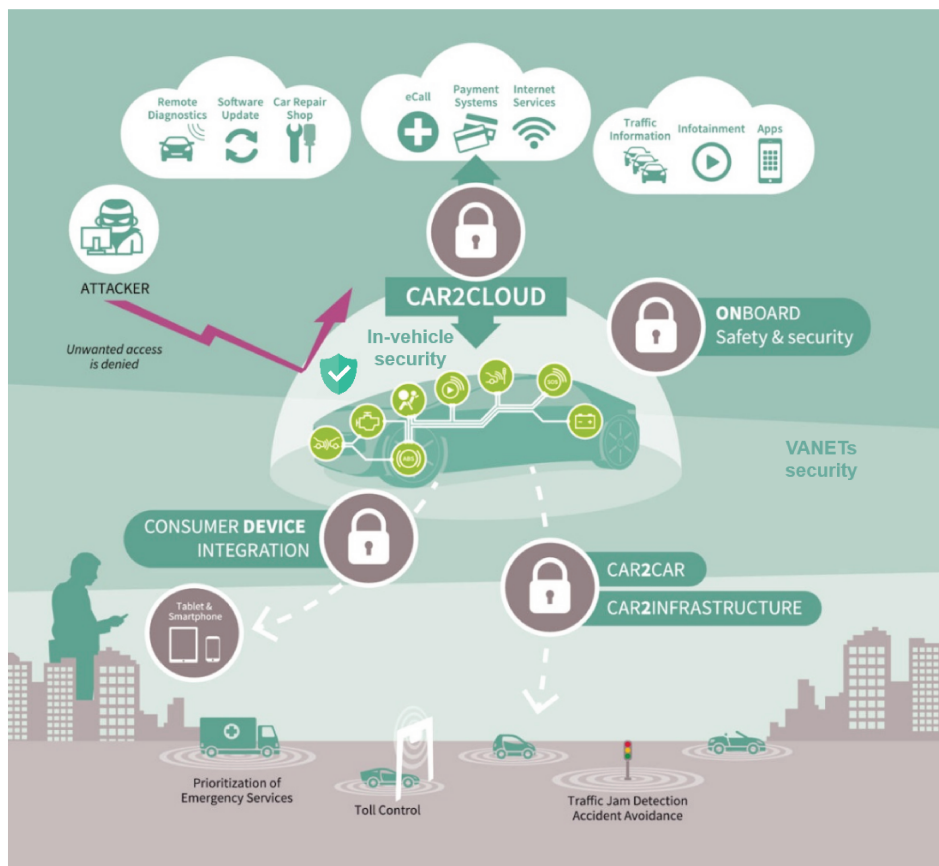
Figure 2.11: In-vehicle network security boundaries Vs VANETs security in the context of intelligent transportation systems.credit CYPRESS (2018)
