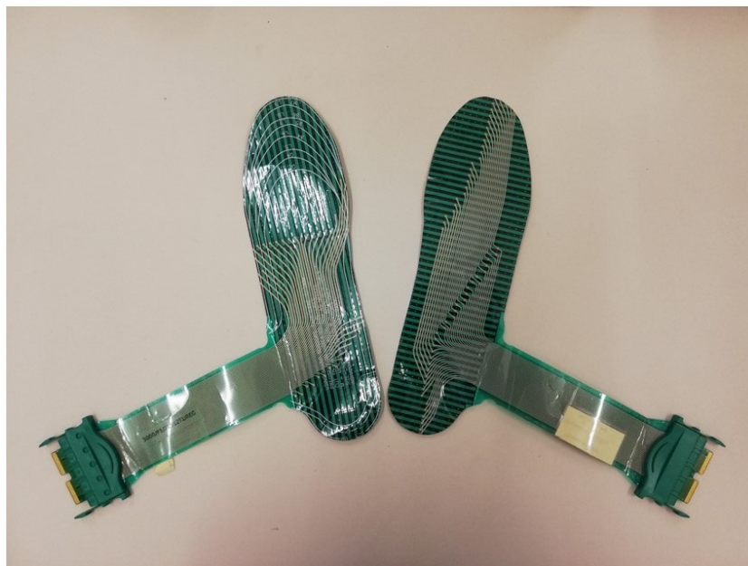
FIGURE 2.16: The Tekscan F-scan Force Sensitive Resistors (FSR) insoles [131]
