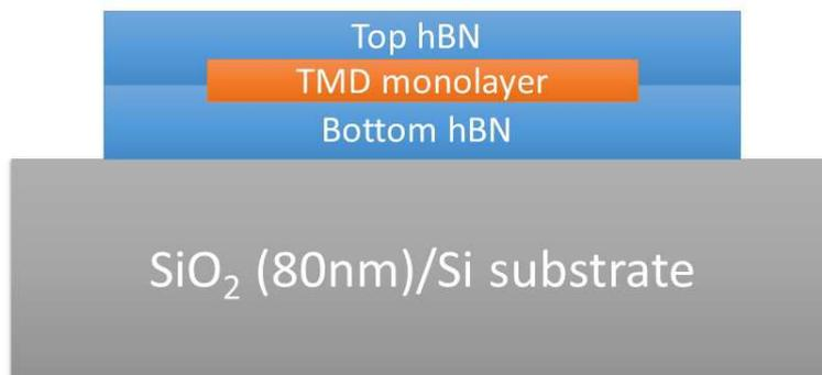
Figure 3.7: Schematic representation of a hBN-encapsulated sample.
