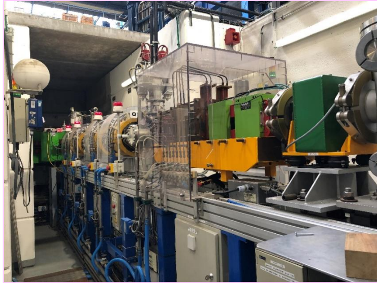
Figure II.6: IRRISUD beamline at GANIL facility. IRRISUD is a low-energy beamline which was used to simulate the effects of high-energy Galactic Cosmic Rays (GCR) on photochemical aerosols deposited on Pluto's surface.
