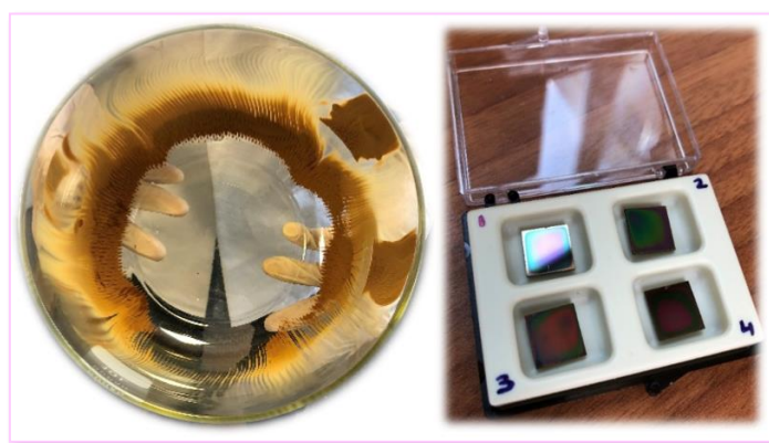
Figure II.4: Pluto tholins synthesized with the PAMPRE experimental setup. Left: Pluto tholins produced as brownish solid spherical grains accumulating in the crystallizing dish. Right: Pluto tholins formed as thin films onto silicon substrates.
