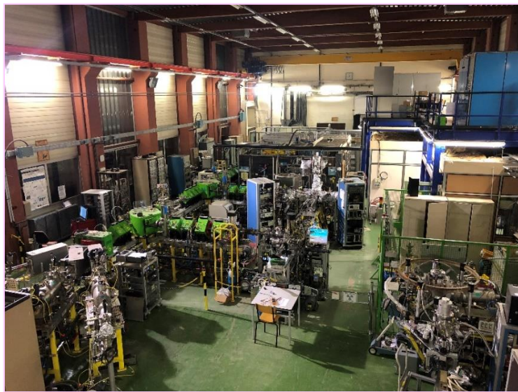
Figure II.7: ARIBE beamline at GANIL facility. ARIBE is a very low-energy beamline which will be used to simulate the effects of low-energy GCR and of Solar Wind (SW) on photochemical aerosols deposited on Pluto's surface.
