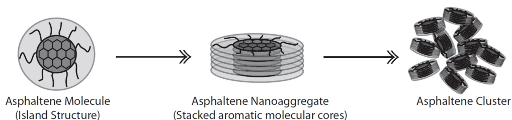
FIGURE 1.12: Schematic of the hierarchical self-association of asphaltenes in good solvents (reprinted from Hoepfner 28 )
