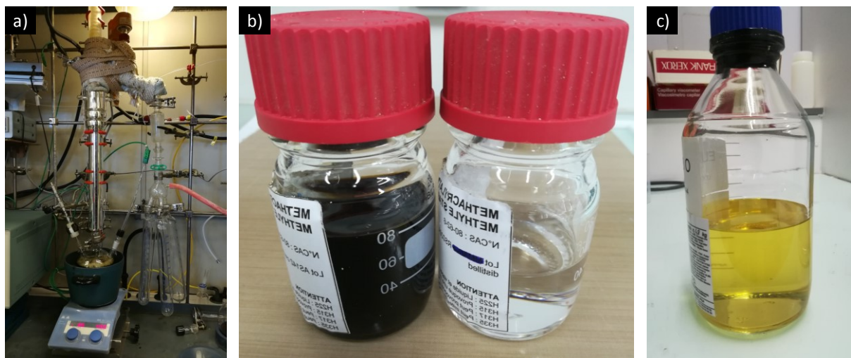
Figure 3-4: (a) Used vacuum distillation setup, (b) distillation input liquid (dark) and distillate (transparent) and (c) Recycled Elium 188-O (rElium) resin obtained from polymerisation of recycled MMA
