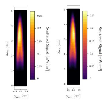
**Figure 7.15:** Synthetized image of scattered signal obtained on the observer. Wavelength: 405 nm. Angle:  $\alpha_o = -40^\circ$  (left),  $\alpha_o = 40^\circ$  (right).
