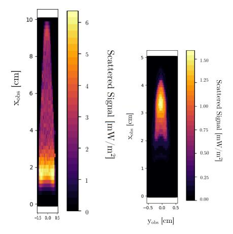
**Figure 7.25:** Synthetized image obtained on the observer : scattering of particles at 405 nm,  $\alpha_o = 0^\circ$ . Top : detailed chemistry, bottom : tabulated chemistry.
