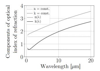
**Figure 4.9:** Evolution of optical index component for soot particles with the wavelength.
