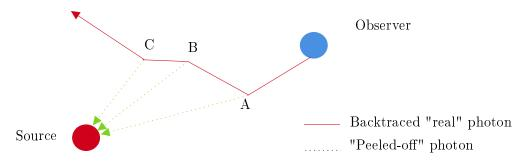
**Figure 7.3:** Principle of peel-off illustrated with a photon scattered three times (points A, B, C). At each scattered location, an additional ray is generated and is traced towards the source.
