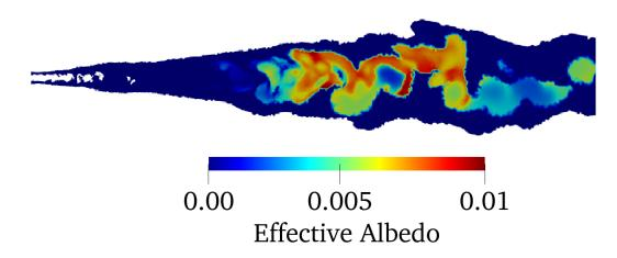
**Figure 3.22:** Computed effective albedo importance  $\overline{\omega}^{eff}$  on the Sandia turbulent jet flame.
