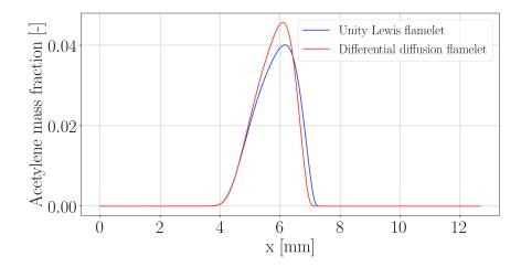
**Figure 5.4:** Comparison of 1D profiles of acetylene mass fraction with/without differential diffusion effects using detailed chemistry (KM2 mechanism) on a 1D counterflow diffusion flame for a strain rate  $a = 100 \text{ cm}^{-1}$ .
