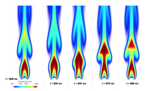
**Figure 7.31:** Flickering behaviour of the laminar flame investigated in Chapter 6 without including radiation.
