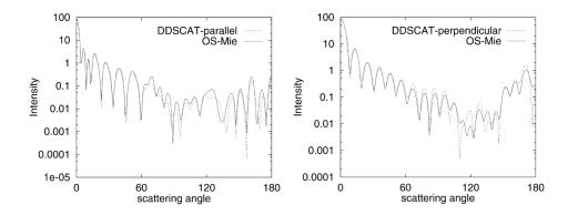
**Figure 1.12:** Comparison of DDSCAT code using DDA and GMM method (from Comberg and Wriedt (1999)) in terms of intensity in a row parallel (left) and perpendicular (right) to an incident electromagnetic wave.
