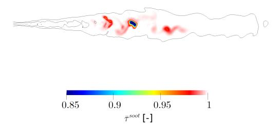
**Figure 3.20:** Mean soot transmissivity  $\bar{\tau}^{soot}$  for the studied turbulent jet flame field. The black line corresponds to an isocontour of Temperature equals to 1000 K. The characteristic length is chosen equals to 0.01 m.
