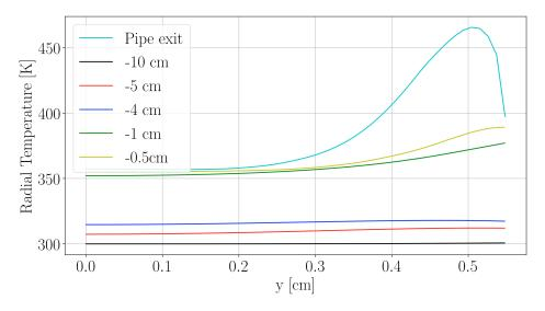
**Figure 6.21:** Radial temperature profiles obtained at various locations along the pipe when accounting for fuel preheating (CHT). The referred positions are relative to the exit of the pipe.
