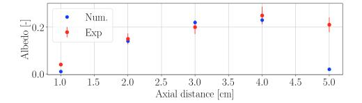
**Figure 6.32:** Reconstructed albedo of aggregates at various heights above the burner with experimental data comparison at 513nm. Errors bars are taken from Iyer et al. (2007).
