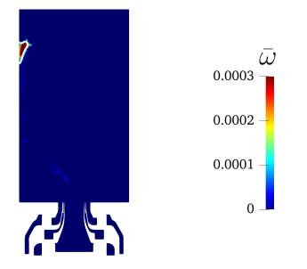
**Figure 4.6:** Computed Scattering Importance metric on the DLR FIRST Combustor chamber. The contour in white represents the zone where the NDF of the 17<sup>th</sup> of the sectional model is maximum.
