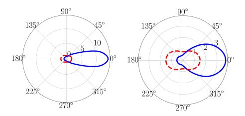
**Figure 7.30:** Computation of phase functions for the thesis computation (left) and detailed chemistry simulation (right) in a polar diagram. The phase function predicted by Rayleigh theory is indicated by a red dashed line.
