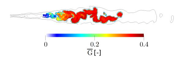
**Figure 3.21:** Mean asymmetry factor  $\overline{G}$  for the studied turbulent jet flame field. The black line corresponds to an isocontour of temperature at 1000 K.
