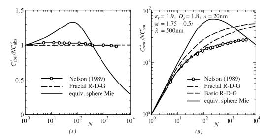
**Figure 1.11:** Comparison of ICP method, RDG standard and for fractal aggregates theories and equivalent sphere Mie method in terms of non-dimensionnal absorption (a) and scattering (b) coefficients. N is the number of soot particles in the aggregate.
