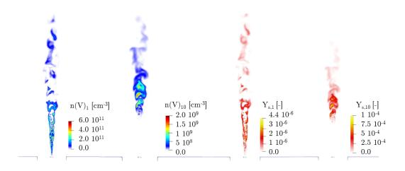
Figure 3.7: Soot mass fraction and soot number density fields for the first and tenth sections.
