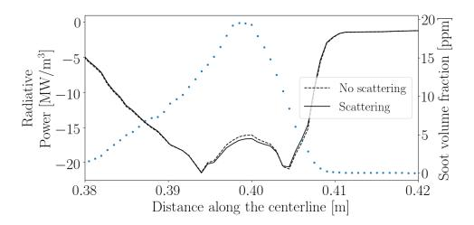
**Figure 3.13:** Comparison of radiative power profiles (left axis, solid and dashed lines) along the jet flame centerline. The plotted region corresponds to the peak in soot volume fraction (right-axis, dotted line).
