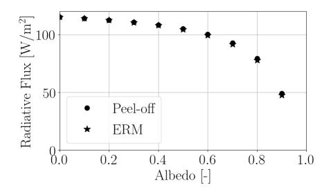
**Figure 7.7:** Radiative flux at the observer as function of the albedo for the ERM  $((\bullet))$  and peel-off  $(\star)$  methods in the case of an homogeneous and isotropic medium  $(\kappa L = 0.01)$ .
