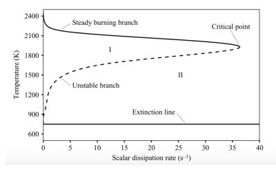
**Figure 5.1:** Schematic "S-curve" representing the set of steady flamelet solutions (solid and dashed black lines), extracted from Pierce and Moin (2004).
