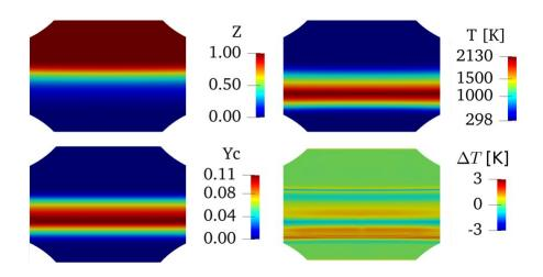
**Figure 5.12:** Obtained fields on the counterflow diffusion flame computed in AVBP. The strain rate is set at  $120s^{-1}$ .
