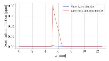
**Figure 5.6:** Comparison of 1D profiles of soot volume fraction with/without differential diffusion effects using detailed chemistry (KM2 mechanism) on a 1D counterflow diffusion flame for a strain rate  $a = 100 \text{ cm}^{-1}$ .
