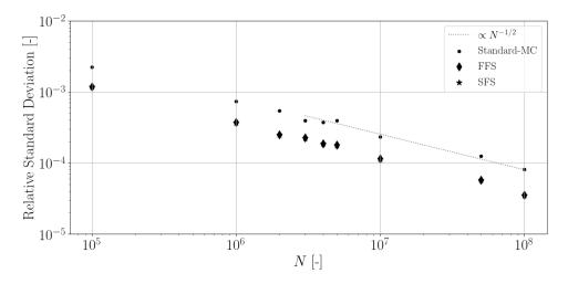
**Figure 2.6:** Relative standard deviation of computed wall emittance as a function of the total number of rays N for standard Monte Carlo case and Standard Forced Scattering and Fast-forced-scattering case. Conditions:  $\tau_L = 0.1$  and  $\omega = 0.9$ . Convergence rate is also displayed in dashed lines.
