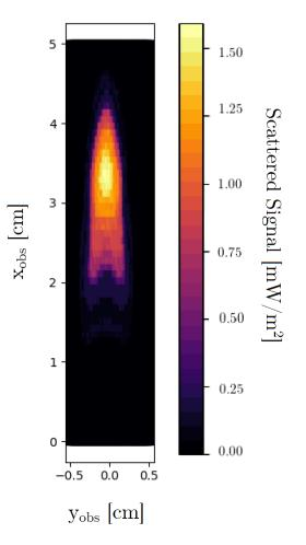
**Figure 7.14:** Synthetized image of scattered signal obtained on the observer. Wavelength: 405 nm. Angle:  $\alpha_o = 0^\circ$ ..
