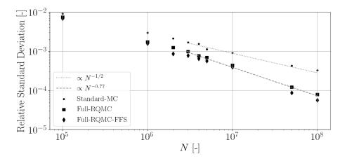
**Figure 2.7:** Comparison of relative standard deviation for the computed wall emittance as a function of the total number of rays N for the cases full-RQMC and full-RQMC-FFS. Conditions:  $\tau_L = 1$  and  $\omega = 0.7$ . Convergence rate is also displayed in dashed lines.
