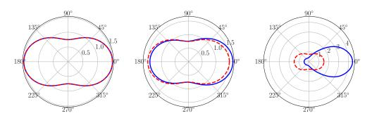
Figure 3.1: Comparison of phase functions between Rayleigh theory (red dashed lines) and RDG-FA theory (blue line) for a given aggregate with 3 different primary particle diameters  $d_p = 1$  nm (left), 10 nm (center) and 50 nm (right). The wavelength is fixed at 534 nm.
