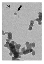
**Figure 1.10:** TEM characterization of soot aggregates for ethylene/air diffusion laminar flame. Both single sphere and aggregates are displayed in the TEM images (Okyay (2016))
