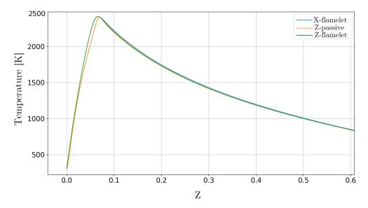
**Figure 5.8:** Evolution of temperature in function of the mixture fraction for X-flamelet and Z-flamelet formulation in a 1D counterflow diffusion flame, accounting for differential diffusion effects.
