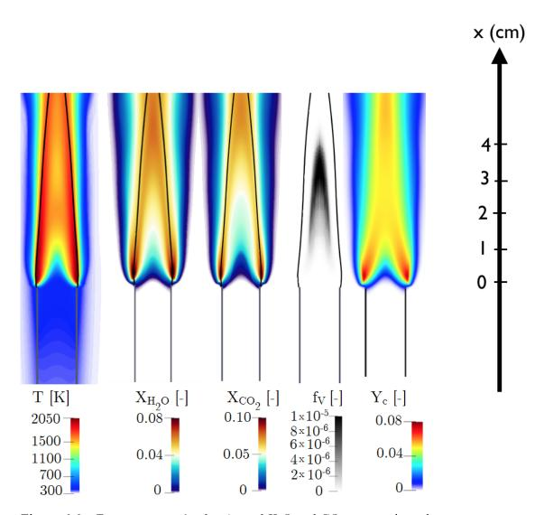
**Figure 6.8:** Temperature, molar fractions of  $H_2O$  and  $CO_2$ , soot volume fraction, and progress variable results from the coupled simulation. The contour Z = 0.064 is also displayed in black line.
