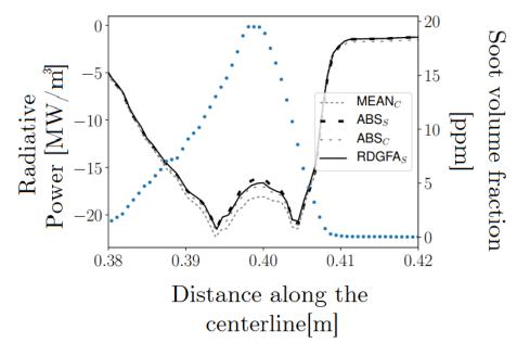
**Figure 4.12:** Radiative power along the centerline of Sandia turbulent jet flame for the 4 considered soot radiative models. Soot volume fraction is represented with dot lines.
