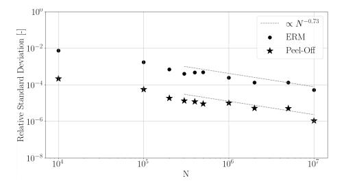
**Figure 7.9:** Relative standard deviation of the computed scattered flux as a function of the total number of rays N for the ERM  $((\bullet))$  and the peel-off  $(\star)$  methods. The fitted convergence rate is depicted by dashed lines.
