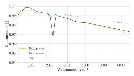
**Figure 6.29:** Impact of soot optical index formulation on the computed transmissivities and comparison with experimental data.
