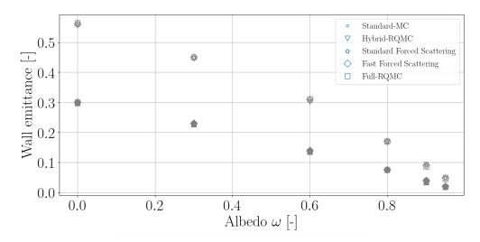
**Figure 2.3:** Wall emittances obtained in function of the albedo  $\omega$  for two optical thickness  $\tau_L$  and for four different scattering treatments. Comparison with reference results from Siegel (1987) is also provided. Plain markers :  $\tau_L = 0.2$ , empty markers :  $\tau_L = 0.5$ .
