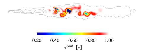
**Figure 4.17:** Mean soot transmissivity  $\bar{\tau}^{soot}$  for the studied turbulent jet flame field with increased particle size. The black line corresponds to an isocontour of Temperature equals to 1000 K. The characteristic length is chosen equals to 0.01 m.
