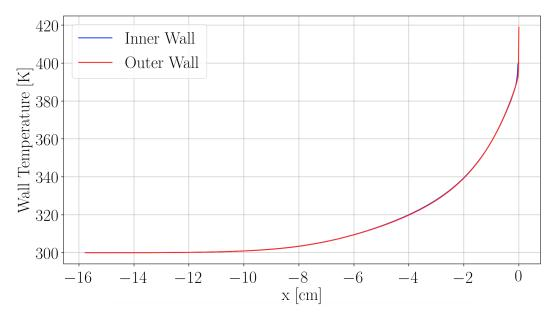
**Figure 6.20:** Obtained wall temperature profiles for the inner, outer and lip walls, accounting for conjugate heat transfer.
