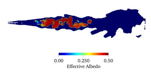
**Figure 4.16:** Mean effective albedo importance  $\overline{\omega}^{eff}$  for the studied turbulent jet flame field with increased particle size.
