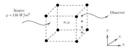
**Figure 7.6:** Peel-off validation case: uniform slab with absorption coefficient  $\kappa$  and albedo  $\omega$ ; the source is defined on the left of the cube with an imposed surface flux; the observer elements are placed along the right face of the cube.
