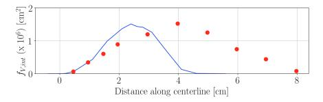
**Figure 6.13:** Integrated soot volume fraction distribution along the axis height above the burner : experimental data from Santoro et al. (1983) ( $\bullet$ )
