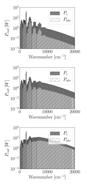
Figure 4.7: Spectral emitted and absorbed radiative power integrated over the volume of the combustion chamber, at P = 3 bars, and with a soot volume fraction multiplied by 10, 100 and 1000.
