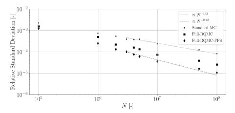
**Figure 2.8:** Comparison of relative standard deviation for the computed wall emittance as a function of the total number of rays N for the cases full-RQMC and full-RQMC-FFS. Conditions:  $\tau_L = 0.1$  and  $\omega = 0.9$ . Convergence rate is also displayed in dashed lines.
