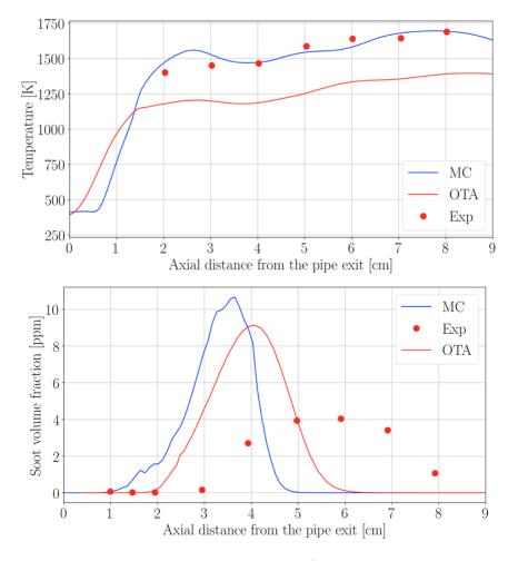
**Figure 6.14:** Comparison Coupled Calculation / optically thin assumption on the predicted soot volume fraction along the centerline and temperature. Experimental data (( $\bullet$ )) from Santoro et al. (1983).
