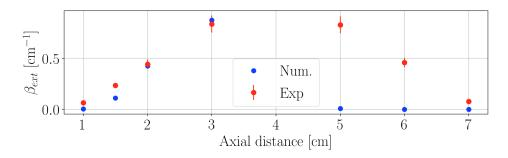
**Figure 6.31:** Axial evolution of the extinction coefficient at wavelength  $\lambda = 513nm$ . Experimental values with associated errors are also reported.
