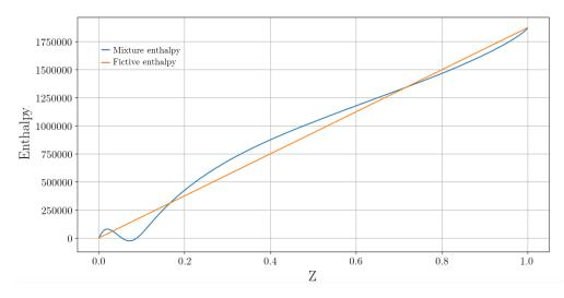
**Figure 5.10:** Evolution of the transported enthalpy and the mixture enthalpy in function of Z for one of the 1D counterflow flamelets generated with the KM2 mechanism for the ethylene
