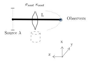
Figure 7.21: Considered ray for the study of the spectral optical thickness evolution.
