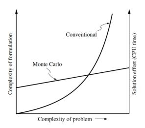
**Figure 1.2:** Comparison between Monte Carlo and other techniques conventionally used for the RTE solutions (extracted from Modest (2003b))
