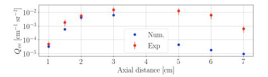
**Figure 6.30:** Axial evolution of the vertical-vertical scattering coefficient (for an angle of  $\theta_i = 90^\circ$  and a wavelength  $\lambda = 513nm$ . Experimental values with associated errors are also reported.
