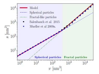
**Figure 4.10:** Derivation of the surface-volume model (SV-1) based on numerical results obtained on 1D laminar premixed flames by Mueller et al. (2009), Salenbauch et al. (2015). Extracted from Rodrigues (2018)
