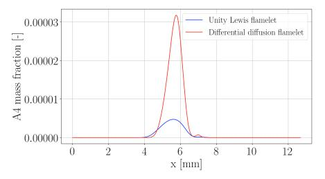
**Figure 5.5:** Comparison of 1D profiles of A4 PAH mass fraction with/without differential diffusion effects using detailed chemistry (KM2 mechanism) on a 1D counterflow diffusion flame for a strain rate  $a = 100 \text{ cm}^{-1}$ .
