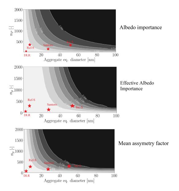
**Figure 7.33:** Evolution of  $\bar{\omega}$  (top),  $\bar{\omega}^{eff}$  (middle) and  $\bar{G}$  (bottom) for various aggregate morphology. The four studied cases in this thesis are indicated with red stars.
