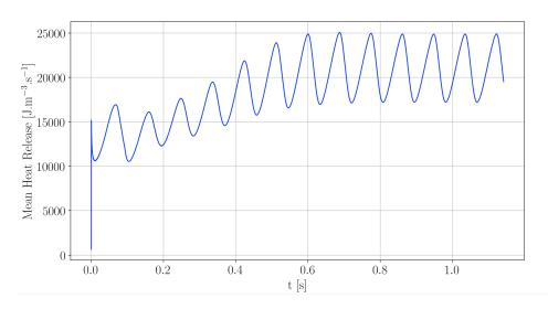
Figure 7.32: Evolution of the heat-release rate in the case of the flickering flame.
