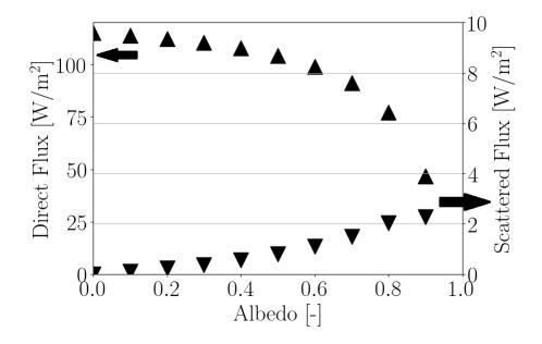
**Figure 7.8:** Radiative flux direct ( $\blacktriangle$ ) and scattered ( $\blacktriangledown$ ) contributions computed with the peel-off methods in the case of an homogeneous and isotropic medium ( $\kappa L = 0.01$ ).
