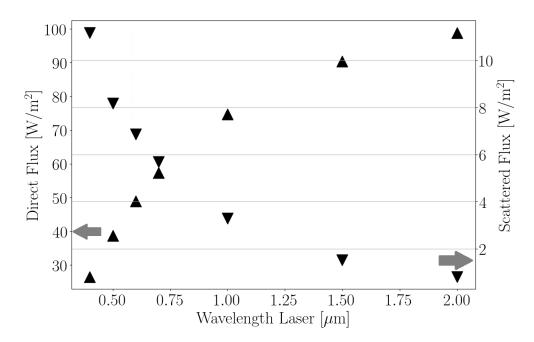
**Figure 7.11:** Radiative flux direct ( $\blacktriangle$ ) and scattered ( $\blacktriangledown$ ) contributions at the observer as a function of the source wavelength for the ERM and Peel-off methods in the case of anisotropic scattering due to soot particles.
