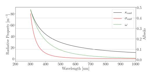
**Figure 7.22:** Spectral evolution of soot radiative properties averaged on a characteristic optical path along the flame.
