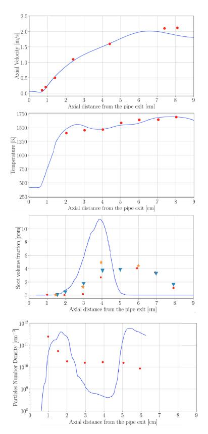
**Figure 6.12:** Centerline profiles of temperature, axial velocity, soot volume fraction and  $N_{part}$  with comparison to experimental data : Santoro et al. (1983) (•), Köylü et al. (1997) ( $\checkmark$ ), McEnally et al. (1997) ( $\star$ ).
