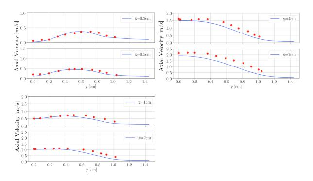
**Figure 6.16:** Comparison of axial velocity profiles for six axial heights above the burner with experimental data from Santoro et al. (1983)  $(\bullet)$ .
