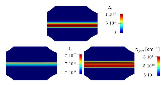
**Figure 5.14:** Obtained fields on the sooty counterflow diffusion flame computed in AVBP. The strain rate is set at  $120s^{-1}$ .
