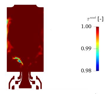
**Figure 4.4:** Soot contribution to the mean transmissivity  $\bar{\tau}^{soot}$  calculated using soot optical properties. The reference length is here chosen equals to 0.01 m. See Chapter 3 for more details on this metric.
