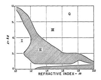
Figure 1.9: Contour error in terms of  $Q_{ext}$ . x is the size parameter and m the refractive index Kerker et al. (1963). Region I corresponds to an error of less than 10% between RDG and Mie's theory. Region II corresponds to an error less than 100%, region III corresponds to an error greater than 100%.
