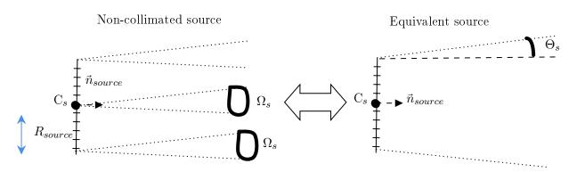
**Figure A.1:** Parametrization of the source for non-collimated radiation : the source is characterized by a deflexion angle  $\Theta_s$ .
