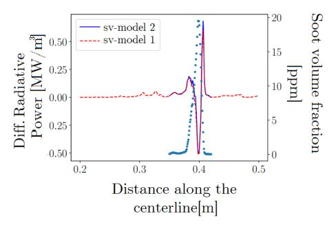
**Figure 4.13:** Difference of radaitive power with and without scattering along the centerline for Sandia jet flame with the two morphological models presented Section 4.3.3. Soot volume fraction is represented with dot lines.
