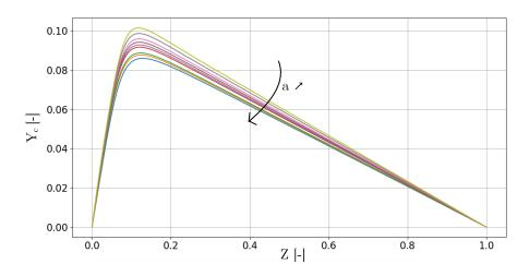
**Figure 5.9:** Evolution of  $Y_C$  in function of Z for different 1D counterflow flamelets generated with the KM2 mechanism for ethylene. Differential diffusion is considered and 2 transported equations for  $Y_c$  and Z are additionally solved. Only the stable branch flamelets are represented.
