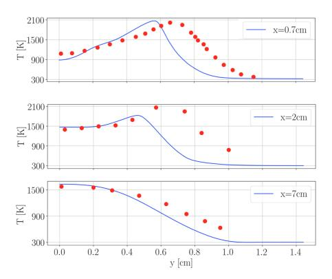
**Figure 6.15:** Comparison of radial temperature profiles obtained for three different axial heights above the burner with experimental data from Santoro et al. (1983) ( $\bullet$ )
