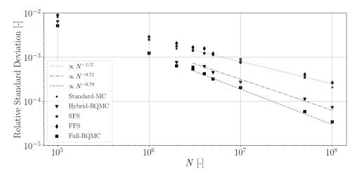
**Figure 2.4:** Relative standard deviation of computed wall emittance as a function of the total number of rays N for the five considered cases. Conditions:  $\tau_L = 0.2$  and  $\omega = 0.3$ . Convergence rates are also displayed in dashed lines.
