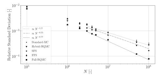
**Figure 2.5:** Relative standard deviation of computed wall emittance as a function of the total number of rays N for the five considered cases. Conditions:  $\tau_L = 1$  and  $\omega = 0.7$ . Convergence rates are also displayed in dashed lines.
