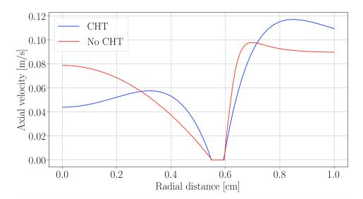
**Figure 6.23:** Comparison between axial velocity profiles at the exit of the pipe, accounting for fuel preheating (CHT) or not. The pipe extends radially between 0 and 0.55 cm, while the coflow extends above 0.59 cm.
