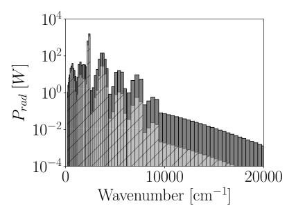
**Figure 4.5:** Spectral emitted and absorbed radiative power integrated over the volume of the combustion chamber.
