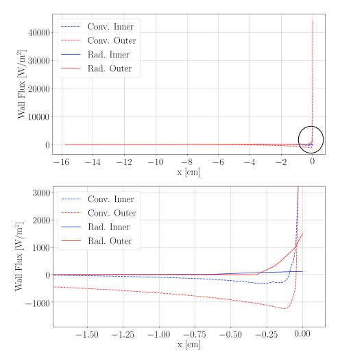
Figure 6.24: Convective and radiative wall fluxes profiles along the inner and outer pipe wall.
