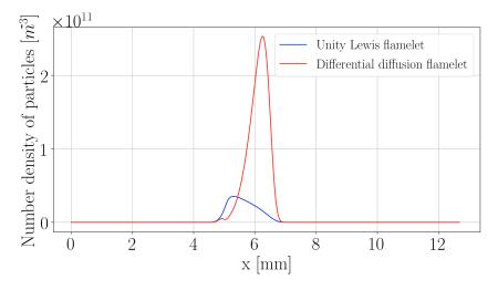
**Figure 5.7:** Comparison of 1D profiles of number density of soot particles with/without differential diffusion effects using detailed chemistry (KM2 mechanism) on a 1D counterflow diffusion flame for a strain rate  $a = 100 \text{ cm}^{-1}$ .
