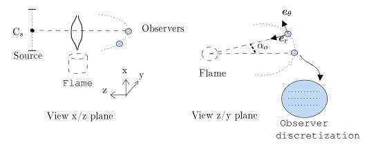
**Figure 7.12:** Parametrization used to generate signals from the Santoro laminar diffusion flame. Left : side view, right : top view.
