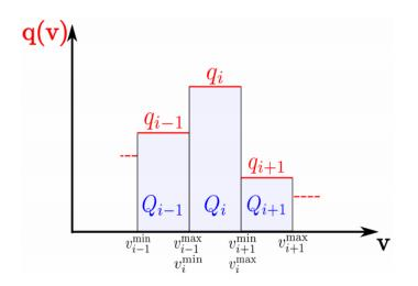
**Figure 1.15:** Discretization of the soot volume fraction density  $q_i(v)$ .
