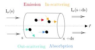
Figure 1.1: Schematic description of radiative mechanisms for the RTE.
