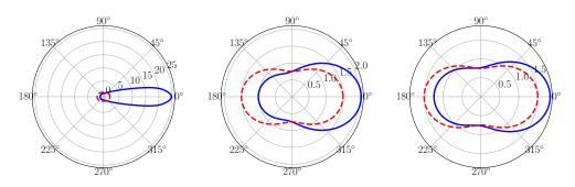
**Figure 3.2:** Comparison of phase functions between Rayleigh theory (red dashed lines) and RDG-FA theory (blue line) for a given aggregate with 3 different wavelengths  $\lambda = 100 \text{ nm}$  (left), 775 nm (center) and 1000 nm (right).
