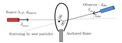
**Figure 7.1:** Schematic of the studied problem: a Laser beam scattered and collected by an observer (2D view). The source and observer are actually much wider.
