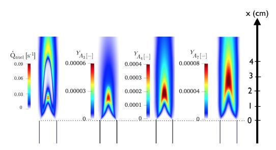
**Figure 6.10:** Mass fraction fields of three PAHs :  $A_3$ ,  $A_4$  and  $A_7$ . The nucleation source term is also displayed on the left.
