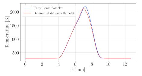
**Figure 5.3:** Comparison of 1D profiles of temperature with/without differential diffusion effects using detailed chemistry (KM2 mechanism) on a 1D counterflow diffusion flame for a strain rate  $a = 100 \text{ cm}^{-1}$ .
