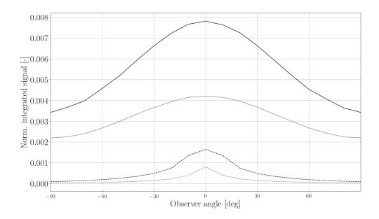
Figure 7.28: Comparison of integrated signals collected by the observer for both computations : thesis work (dashed lines), detailed chemistry (solid lines) at two different wavelengths (405 nm : black, 785 nm : gray).
