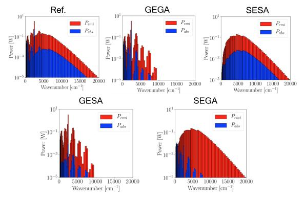
**Figure 6.27:** Spectral emitted and absorbed volume-integrated powers for the instantaneous representative solution. Results correspond to the reference case taking into account gas and soot particles emission and absorption and the four other studied cases: GEGA, GESA, SEGA and SESA.
