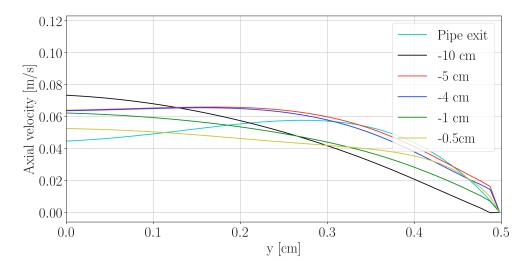
**Figure 6.22:** Radial axial velocity profiles obtained at various locations along the pipe when accounting for fuel preheating (CHT). The referred positions are relative to the exit of the pipe.
