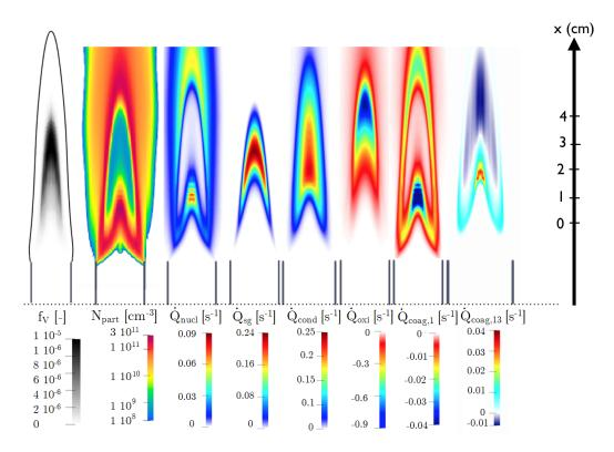
**Figure 6.9:** Soot volume fraction, total particles number density and soot source terms (nucleation, surface growth, coagulation, oxidation and condensation for two sections.)
