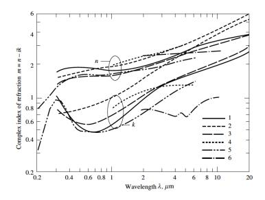
Figure 1.4: Comparison of soot complex index of refraction (from Modest (2003b)). 1 : Lee and Tien (1981) (polystyrene and plexiglas soot), 2 : Stull and Plass (1960) (amorphous carbon), 3 : Dalzell and Sarofim (1969) (propane soot), 4 : Howarth et al. (1966) (pyrographite at 300K), 5 : Chang and Charalampopoulos (1990) (propane soot), 6 :Felske et al. (1984a) (propane soot)
