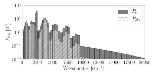
**Figure 4.8:** Spectral emitted and absorbed radiative power integrated over the volume of the combustion chamber at P = 30 bars, obtained with the reference  $f_V$  field.
