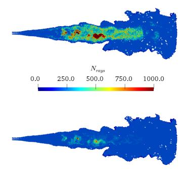
Figure 3.10: Comparison of the number of rays required to reach a given error on the Sandia's turbulent jet flame. Top : Standard-MC, Bottom : full-RQMC-full.
