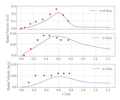
**Figure 6.17:** Comparison of radial velocity profiles for six axial heights above the burner with experimental data from Santoro et al. (1983)  $(\bullet)$ .
