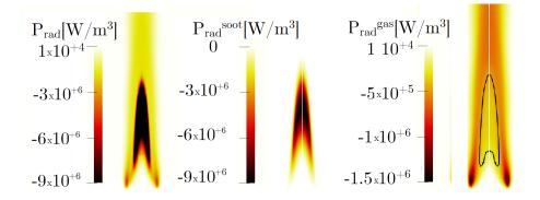
**Figure 6.25:** Participating gases and soot particles contributions to the total radiative power. An iso-contour of  $f_V = 1$  ppm is also displayed on the gaseous phase contribution.
