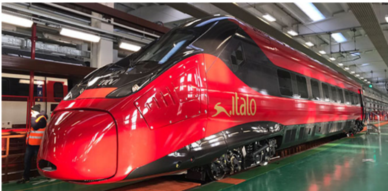
Figure 1.5: Advanced aerodynamic nose of high speed train ETR 675
