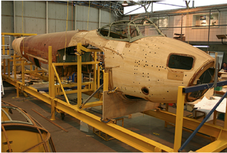
Figure 1.4: Ply-balsa-ply sandwich structure designed for the fuselage of de Havilland DH.98 Mosquito multi-role combat aircraft
