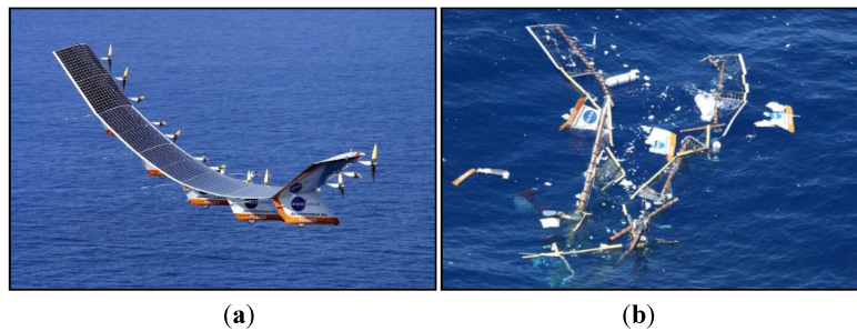
Figure 2: (a) NASA's Helios wing and (b) its wreckage in the Pacific [6]
