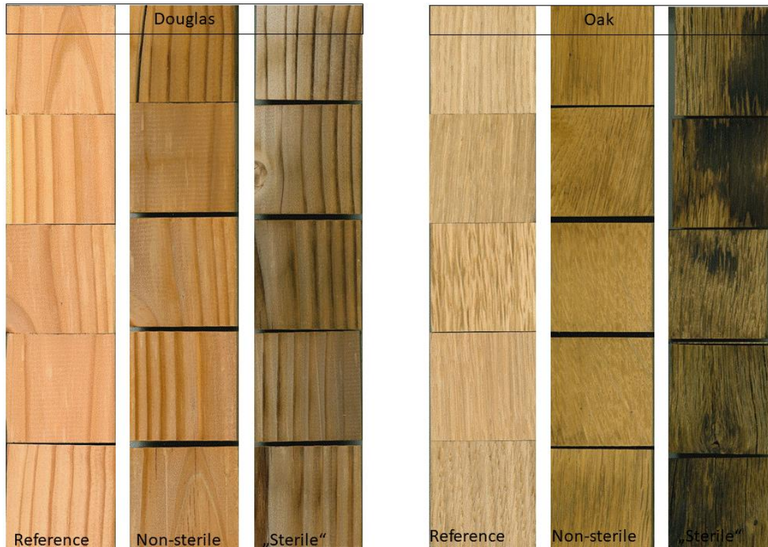
Figure 92: Scans of Douglas and oak specimens before (left), non-sterile (middle) and “sterile” (right) exposure
