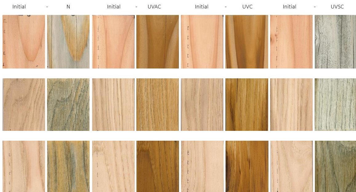
Figure 62: Scans of Douglas (upper row), oak (middle row) and chestnut (third row), NSWE exposed for 12 weeks
