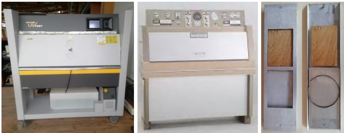
Figure 54: From left to right: Atlas weathering machine with water reservoir and spraying system, Q-lab apparatus, and sample racks to mount the specimens
