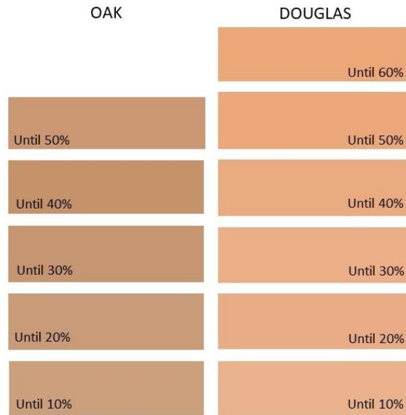
Figure 98: Visual representation of colours for oak and Douglas fir, for the different groups of MC
