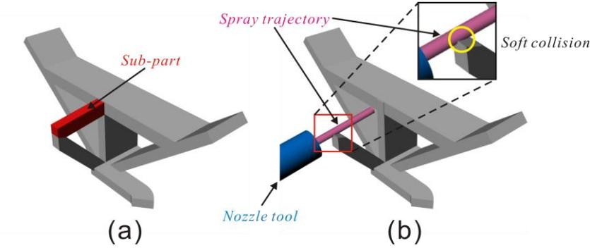
Fig. 4.28. The soft collision in case 3.
