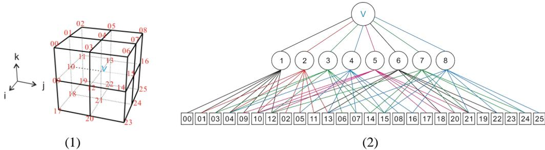
Fig. 3.4. (1). The indices of the 26-neighbourhood of a point  $v$ ,  $N(v)$ ; (2). The adjacency of  $N(v)$ .
