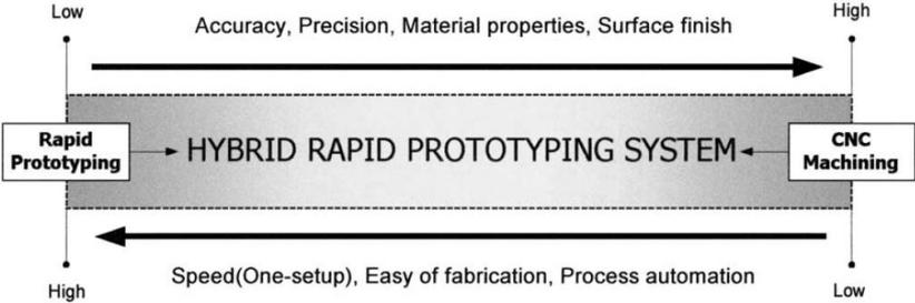
Fig. 1.3. The characteristics of RP and CNC processes [9].
