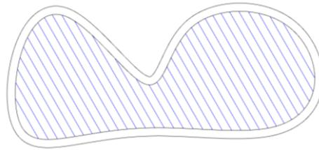
Fig. 3.35. The toolpath strategy: the contour with rastering.
