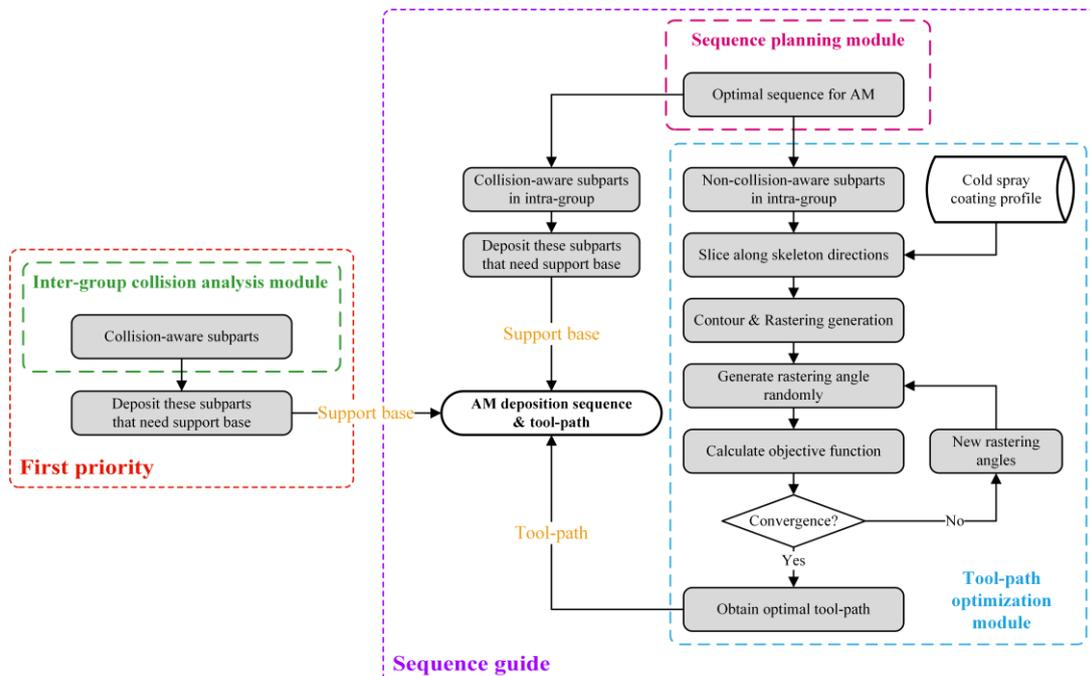
Fig. 3.33. The proposed method for toolpath planning.
