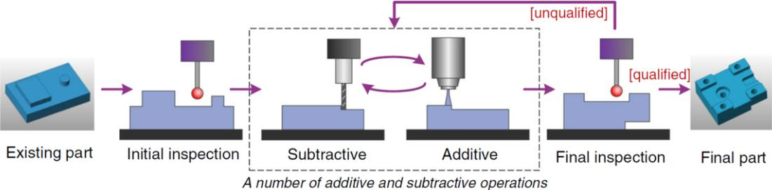
Fig. 2.29. The schematic diagram of the iAtractive process [127].
