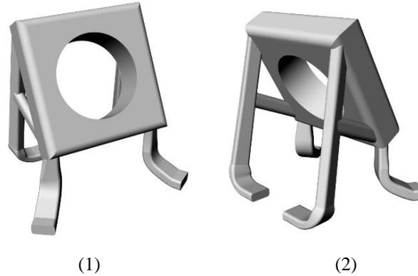
Fig. 4.11. The CAD model of bracket in Rhino.
