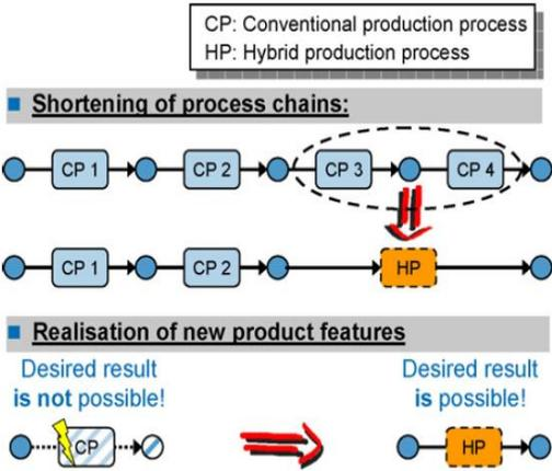
Fig. 1.2. The potential aims of hybrid manufacturing processes [8].
