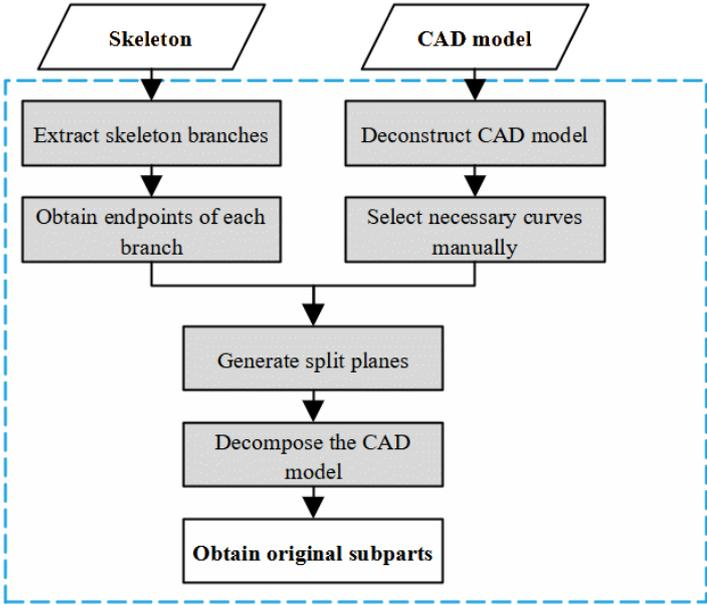
Fig. 3.6. The generation of the original subparts.
