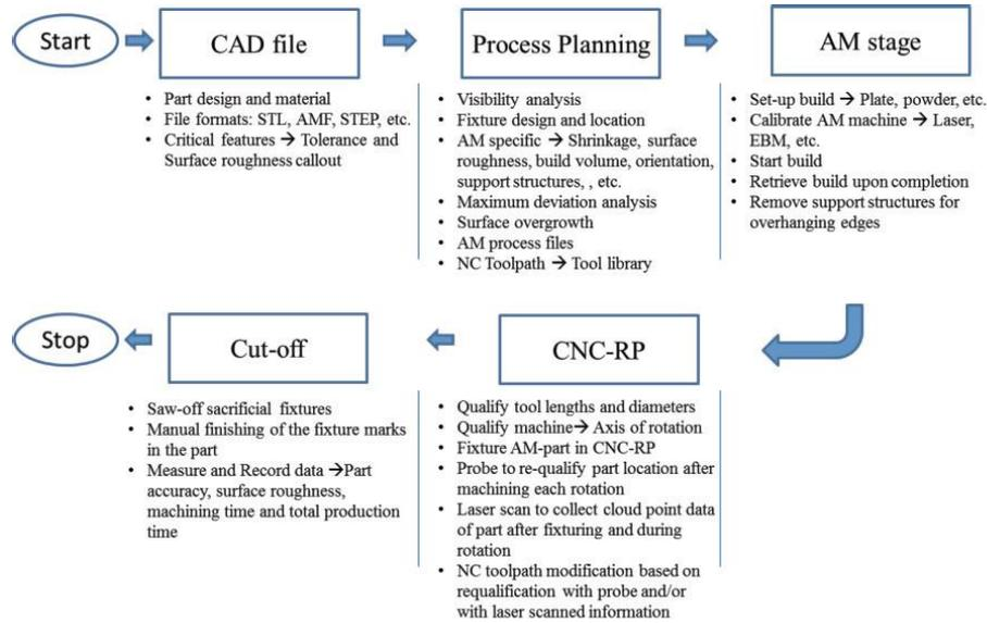
Fig. 2.24. The AIMS process flow [70].
