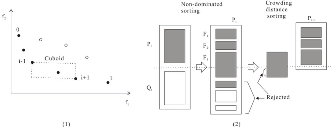
Fig. 3.25. (1). The crowding-distance calculation; (2). The NSGA-II procedure [156].
