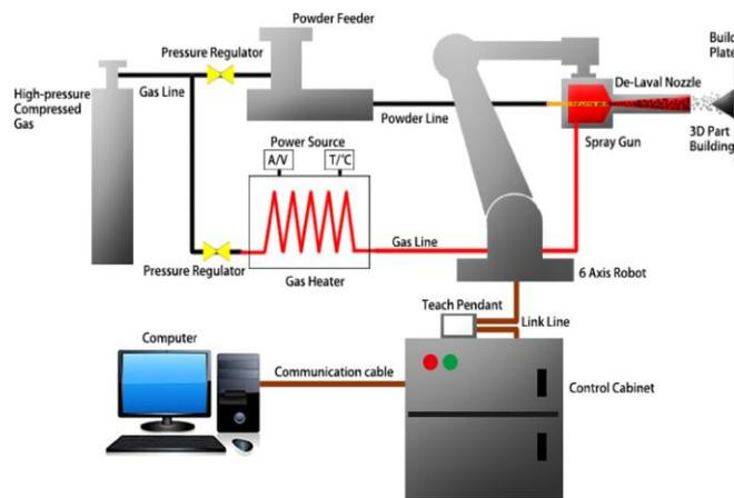
Fig. 1.9. The schematic diagram of the CSAM module [19].
