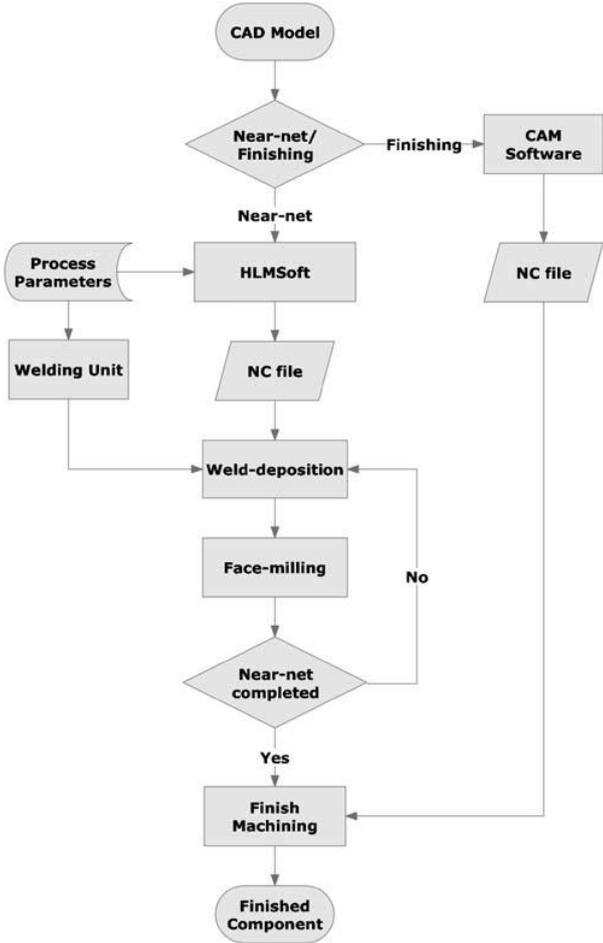
Fig. 2.5. The flow chart for ArcHLM process [43].
