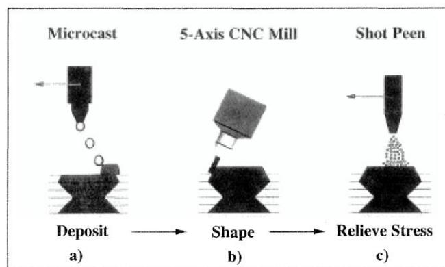
Fig. 2.4. The creation of a layer using SDM [58].
