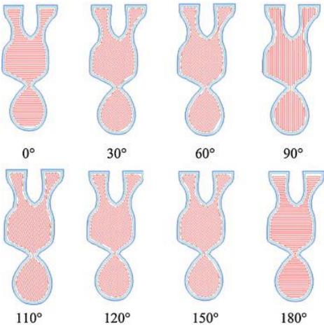
Fig. 2.45. The toolpath with 8 different inclinations [150].
