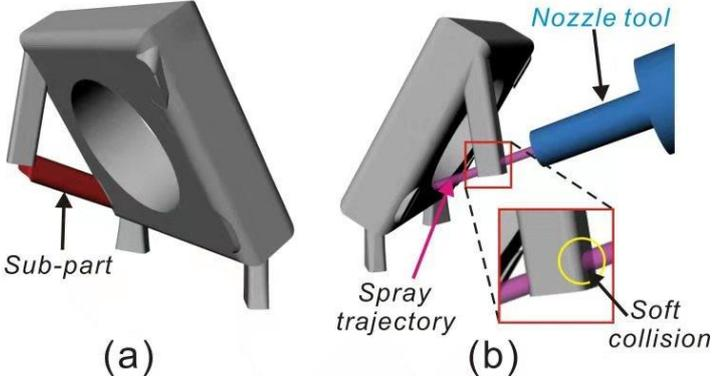
Fig. 4.18. One example of soft collision in case 2.
