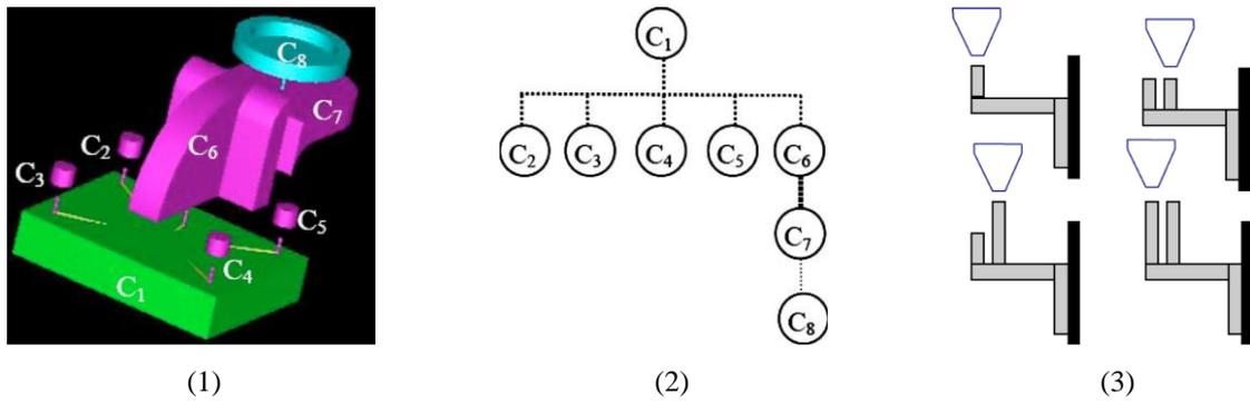
Fig. 2.35. (1). The decomposition; (2). The building relationship graph; (3). The building sequence [126].
