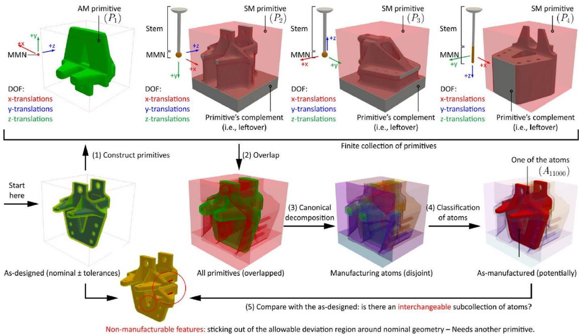
Fig. 2.25. One example including 2 AM and 3 SM primitives [128].
