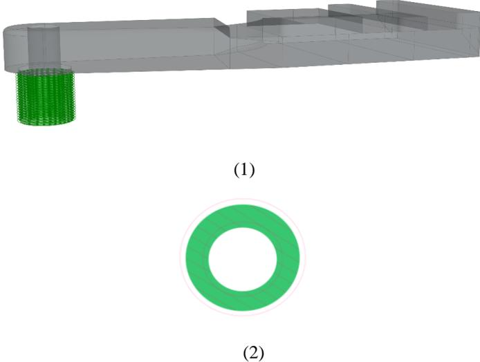
Fig. 4.8. (1). The toolpath of subpart 1; (2). One layer of toolpath of subpart 1.
