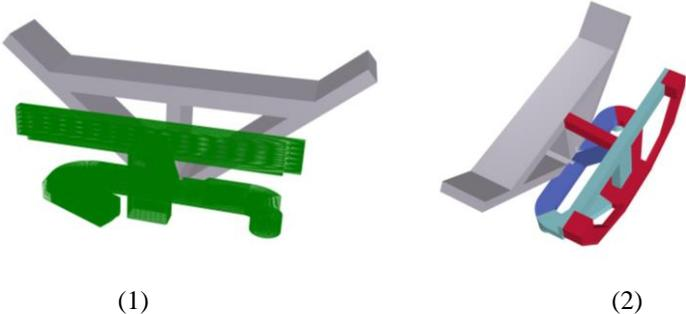
Fig. 4.30. (1). The toolpath of all subparts which do not have collisions in case 3; (2). The subparts that have collisions
