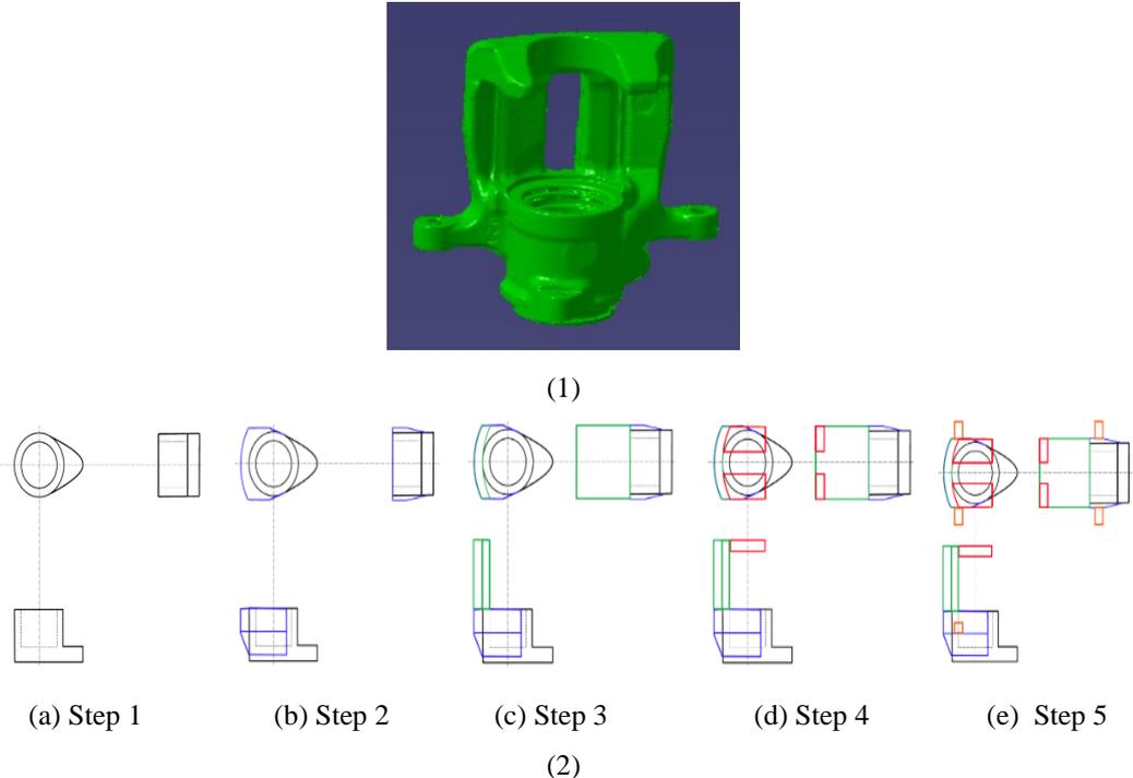
Fig. 1.11. The manual sequence planning according to experiences in an industrial manufacturing process.
