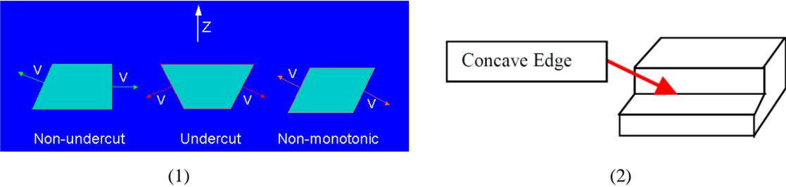
Fig. 2.22. (1). The face classification [5] ; (2) The edge classification [66].
