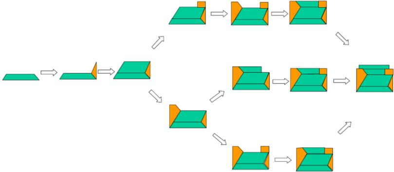
Fig. 2.34. The alternative building sequences [77].
