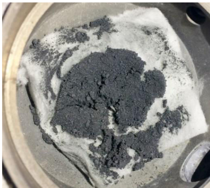
Figure A-6. Iron oxide powder after four cycles at different temperatures.
