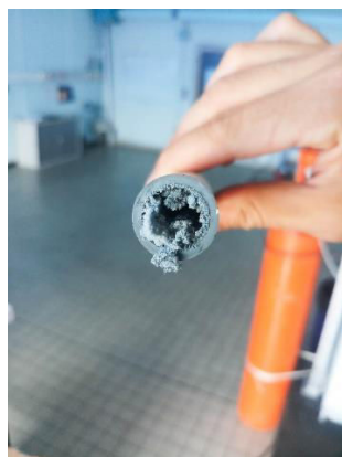
Figure C-7. Crystallized gray chunks (recombined ZnO) located only at the tip of the alumina tube where Zn is condensed (over ~ 1 cm length).
