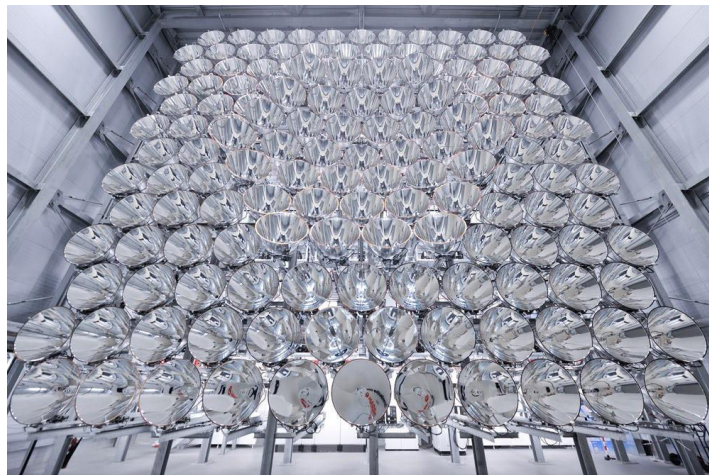
Figure 1-7. 149 xenon short-arc lamps that are employed to simulate solar irradiation at DLR in Jülich, Germany [10].
