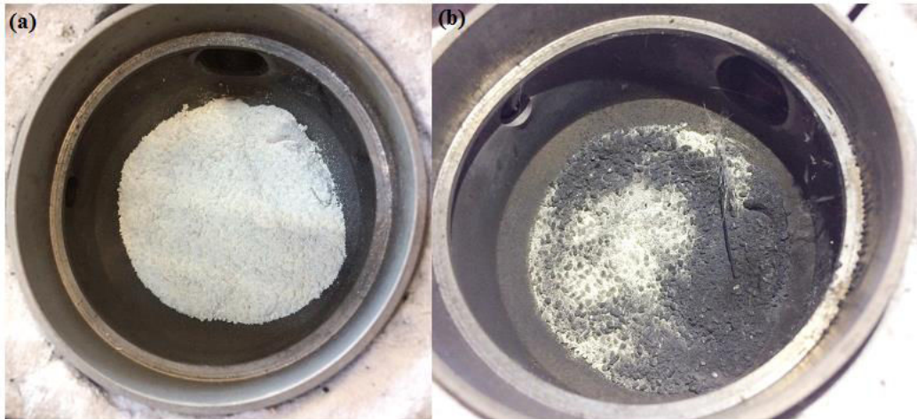
Figure A-13. Ceria powder mixed with Al 2 O 3 particles as dispersion promoter for the solar cavity receiver: (a) before experiments, (b) after experiments for 6 cycles.
