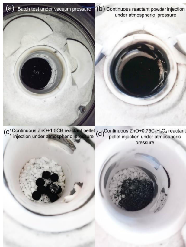
Figure C-6. Carbon remaining in the cavity receiver after experiments: (a) Run. No.1, (b) Run. No.7, (c) Run. No.12, and (d) Run.No.16.
