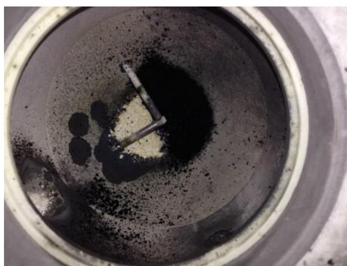
Figure D-3. Char and ZnO remaining inside the cavity of the reactor for a biomass/ZnO molar ratio of 0.5 at 1100 °C.
