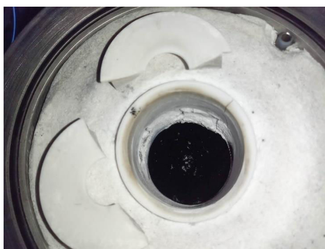
Figure C-18. Carbon remaining in the cavity receiver after experiments (Run. No. 6).
