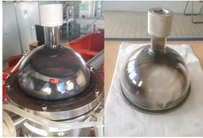
Figure B-3. Dirt deposits on the window observed at low temperature (1100°C).
