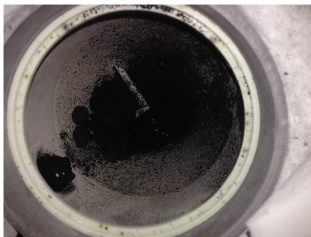
Figure D-5. Char remaining inside the cavity of the reactor for a biomass/ZnO molar ratio of 1 at 1100°C.
