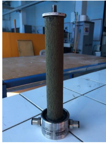
Figure A-12. Carbon deposition on the filter (sample: ceria foam ST-1000, 18.3705 g, cycles: 1-4).
