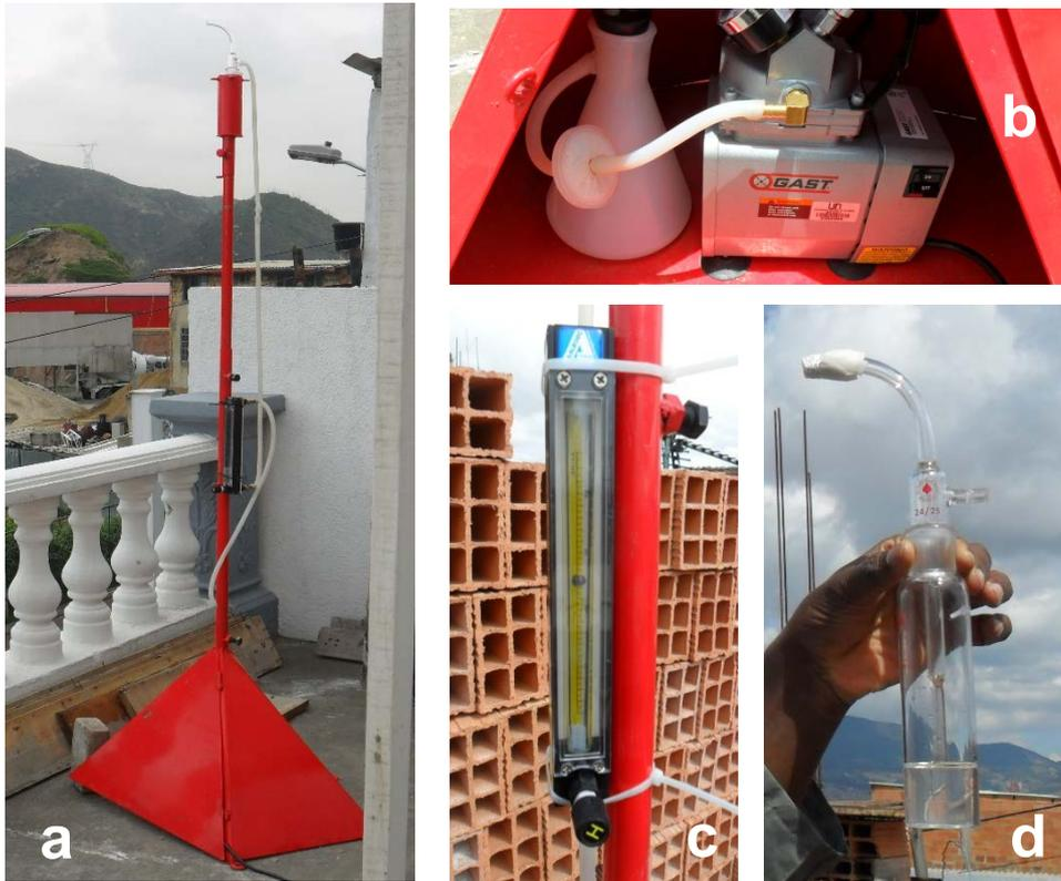
**Photos 1a-d:** Air sampling station used to trap airborne human pathogens: (a) entire air sampling station on the terrace of a house of *Quintas del Plan Social* neighborhood; (b) vacuum pump; (c) flow tube rotameter; and (d) Impinger with PBS.
