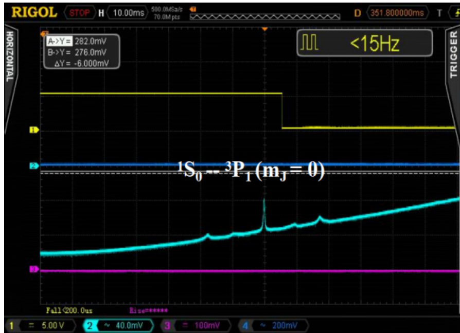
Figure 3.29: Implementing 10 G magnetic field to resolve different m_F states and the crossovers in terms of the 5s5p\ ^3P_1 transition.
