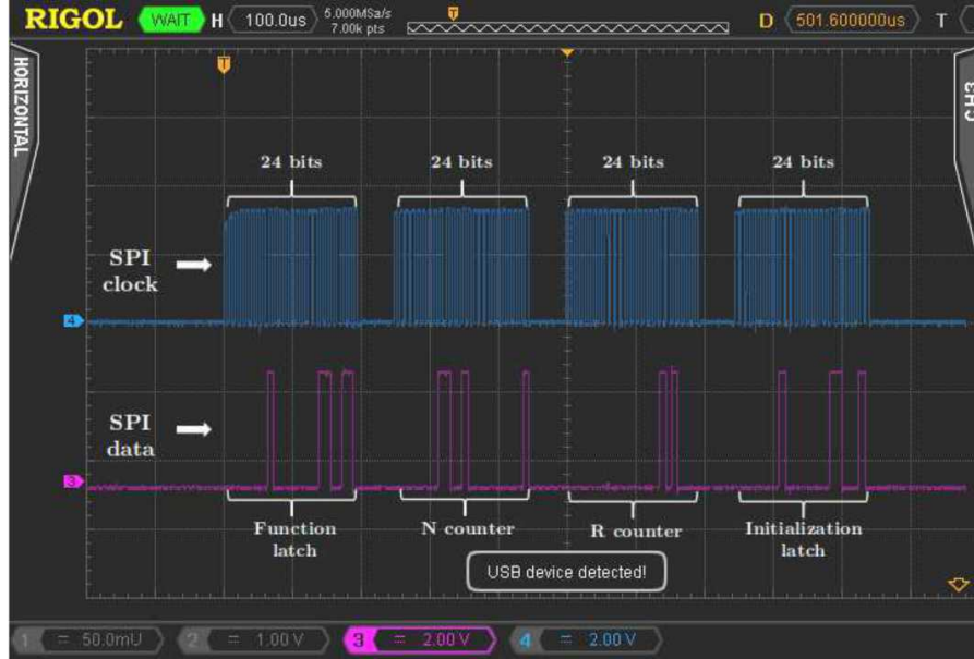
Figure 3.12: SPI timing sequences to configure the PFD.
