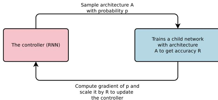
Figure 2.4 **Reinforcement learning approach used in one of the first NAS works.** Figure from (Zoph et al., 2018). States consist of architectures up to current layer. Actions are choices for next layer. The reward is the accuracy obtained if the architecture is complete and 0 otherwise.
