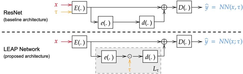
Figure 6.8 **Baseline and LEAP architecture:** Top: ResNet (He et al., 2016) architecture, with  $\tau$  as input. Bottom: Proposed LEAP net:  $\tau$  intervenes in the latent embedding space. The effect is to make a “leap” in latent space.
