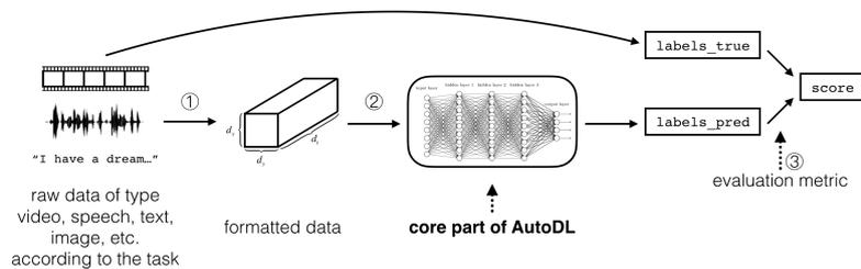
Figure 1.1 **Data flow in AutoDL challenges.** Different types (video, speech, text, etc) of data are first uniformly formatted in a tensor-based format then passed to the core part of AutoDL, which applies one single learning algorithm and tries to maximize the learning performance in terms of an evaluation metric
