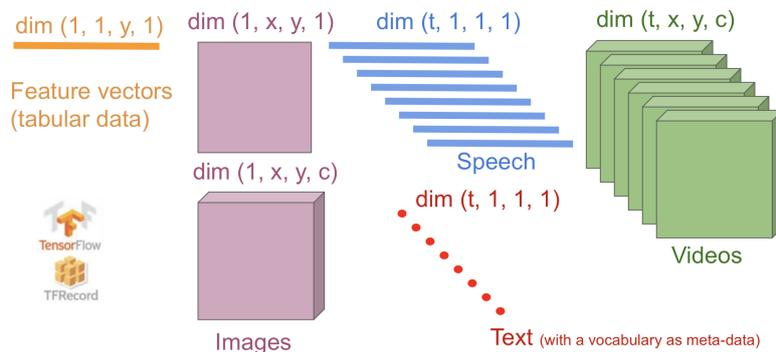
Figure 3.2 **4D-tensor format of the datasets we formatted during this thesis.** This format can encode data for which each example can be an image, a video, a document, an audio or a feature vector. All data are provided *raw* without pre-processing, in TensorFlow (Abadi et al., 2016) TFRecord format.
