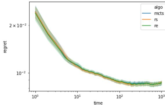
Figure 5.18 **Comparison of NAS methods on NAS-Bench-101 benchmark.** The NAS methods are: our approach (mcts), random search (rs) and regularized evolution (Real et al., 2019) (re). Errors bars are computed over 10 runs. Regret is the difference between the current best obtained test accuracy of the search and the global optimum. Time is in seconds.)
