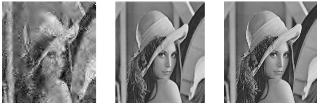
(f) E_b/N_0 = 3 dB UEP, QPSK Adaptive OFDM PSNR = 34.8 dB
