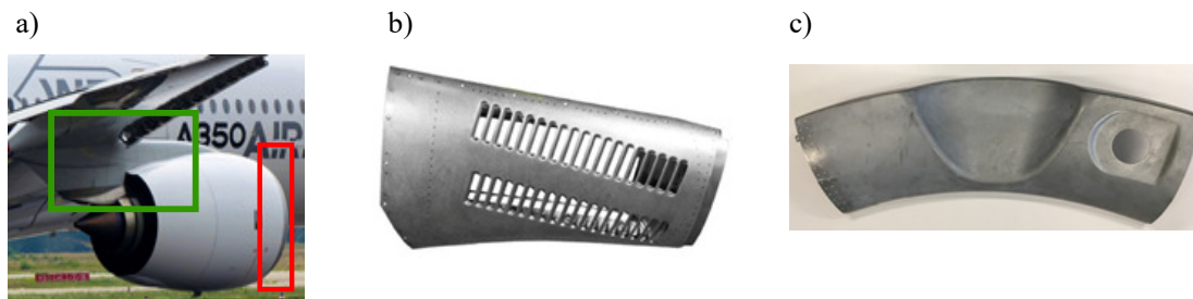
Figure 2: An example of aircraft pieces made of TA6V alloy: (a) in green: engine pylon, in red: engine air inlet, (b) heat exchanger cover in engine pylon fairing (Lauak, 2020), (c) segment of A380 engine air inlet bulkhead (Harvent, 2010)
