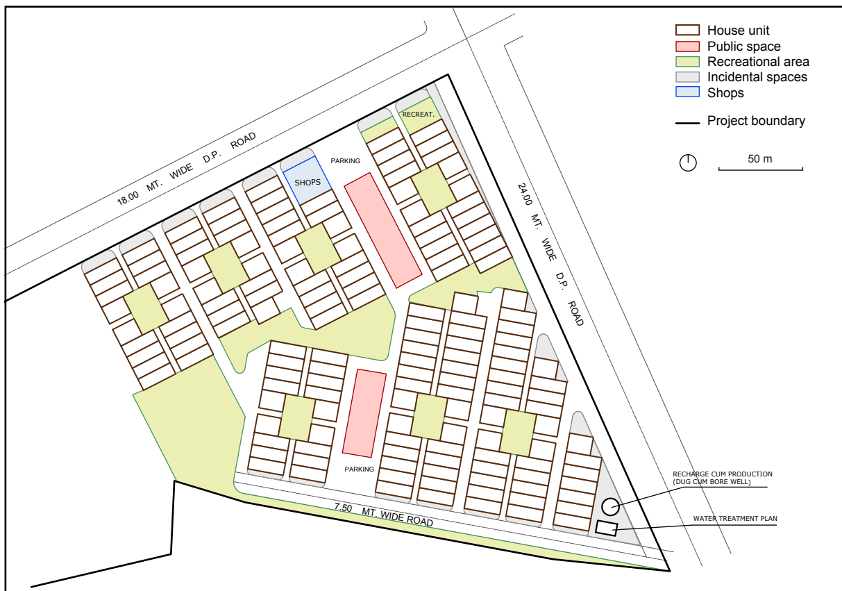
Site Layout for GIDC Relocation Site
