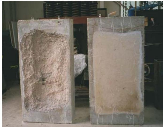
**Figure 3.22** Efficiency of polypropylene fibers against spalling due to fire. On the left: a sample without fibers, on the right: a sample with polypropylene fibers [52].
