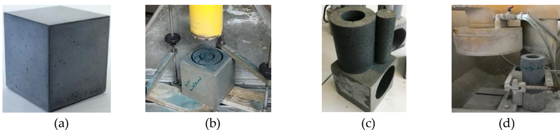
Figure 3.48 Stages of sample preparation : a) concrete cube, b) double coring of sample, c) after coring, d) grinding of the sample.
