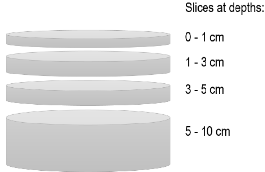
Figure 3.45 Schematic presentation of concrete slices cut for determination of water content at various depths for air-cured samples and water content values determined.
