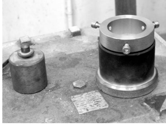
Figure 2.10 Packing fraction using microvibration: mass, container and vibrating table [37].
