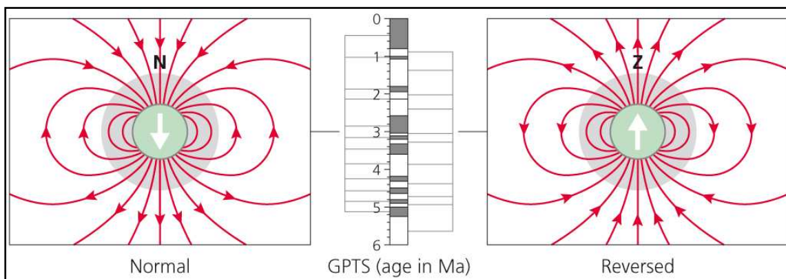
Figure 3.6: The Earth's magnetic field in normal (black) and reverse polarity (white), as recorded in the Geomagnetic Polarity Time Scale (GPTS) (after De Groot & Krijgsman, 2015).
