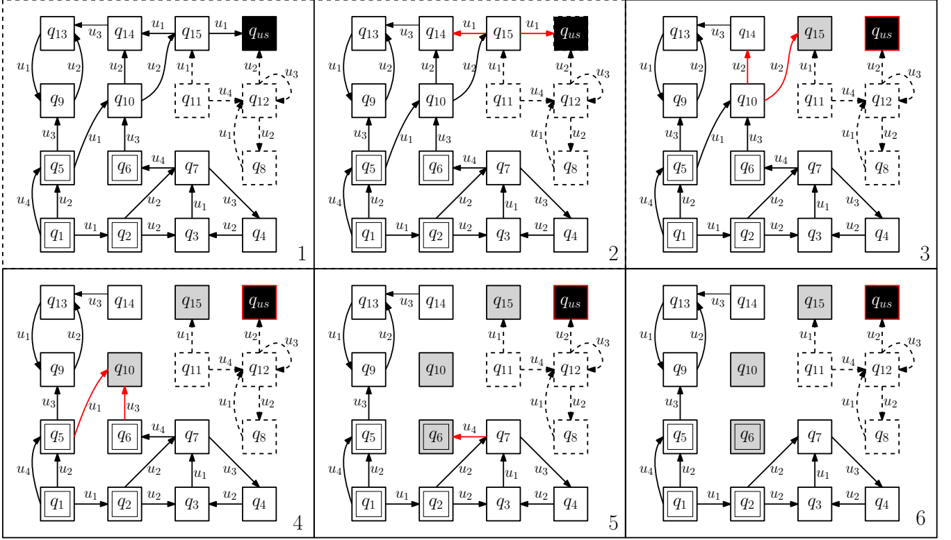
Figure 2.4: Illustration Algorithm 2.4 execution. Unsafe actions are red, blocking states are grey, and the initial states are marked with a double line. The computations are restricted to states, which are reachable from the initial set. States which are non-reachable from the initial set are countered with a dashed line. Hence, states q_{11} , q_{12} and q_8 are not included in the domain of the maximal state lazy safety controller.
