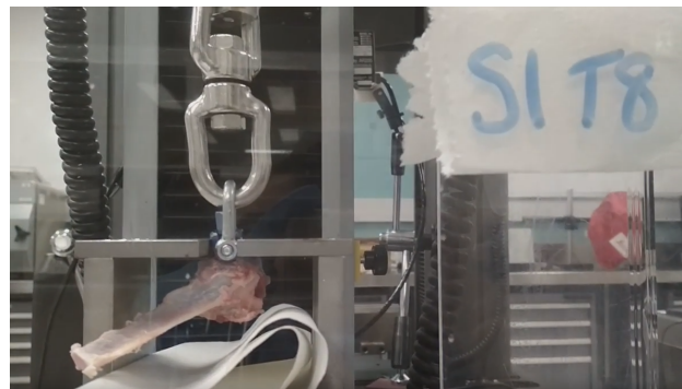
(b) Pull-out test of a vertebral screw in a T8 thoracic sheep vertebra.
