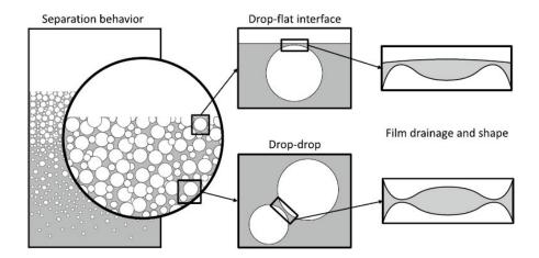
Figure 3: Schematic representation of the separator unit and other important length scales in the system. Reproduced from [9].
