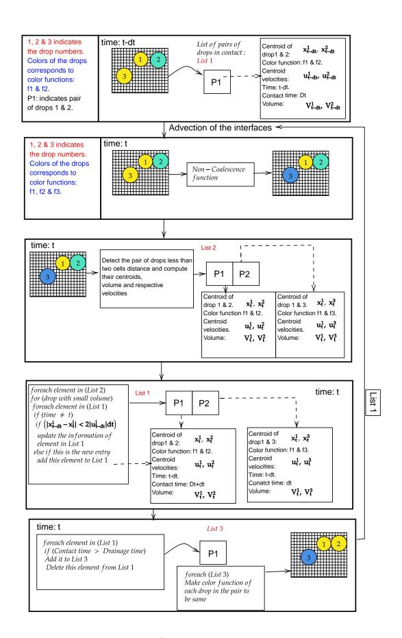
Figure 2.33: Control coalescence algorithm.
