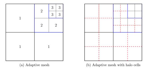
Figure 2.2: Quadtree adaptive grid.
