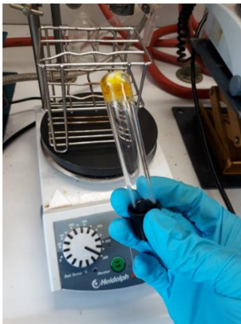
Figure S.IV-2 Strong yellow gel obtained after addition of silane reagent to the catalytic system composed of \text{Cu}(\text{OAc})_2 \cdot x\text{H}_2\text{O} and DTBM-( R )-Segphos ligand.
