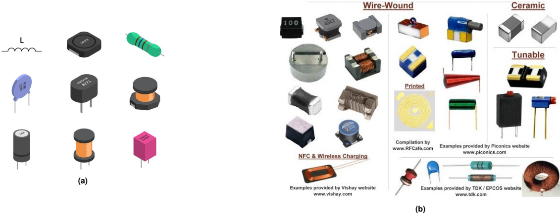
Figure 2.8: Different configurations of inductors. (a) Electronic symbol of inductor, SMD inductors (or inductor chips) and other configurations. (b) Different types of inductors.
