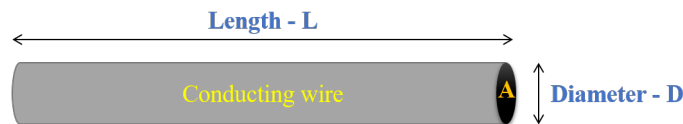
Figure 2.4: Geometry viewpoint of a resistor made up of uniformly conductive wire: A and L are the cross-sectional area and the length of the material respectively.
