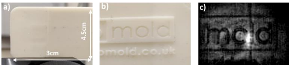
Figure II-12 a) Picture of the object to image b) Hidden text c) Real-time image from the THz camera using the high average power from the cavity PCS showing the hidden text. A real-time video is shown in the supporting content (see visualisation1 ).
