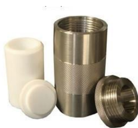
Figure 41 – Image of the Teflon® and autoclave used for the hydrothermal synthesis (www.metalquimica.com).
