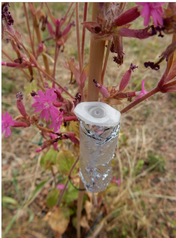
Figure S1: Picture of glass tube with PAA dilution used in the experiment to increase PAA emission.
