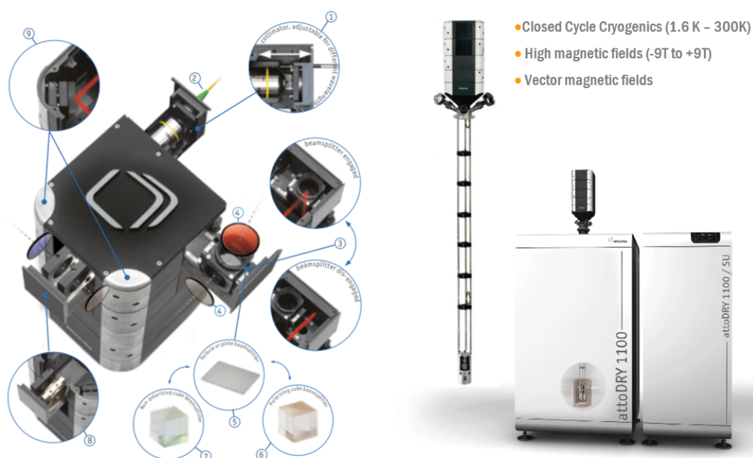
Figure 2.1: The attocube fiber-based confocal microscope attoCFM and attoDRY1100 cryostat. (1) Collimator. (2) FC/APC coupled single mode fiber to/from excitation laser or detector/spectrometer. (3) Beam-splitter position easily switchable from outside. (4) Two additional filter mounts on beam-splitter cube. (5) Beam-splitter options. (6) Optional: polarizing beam-splitter cube. (7) Optional: non-polarizing beam-splitter cube. (8) Filter drawer. (9) Theta/phi mirrors for each channel easily adjustable from the outside.
