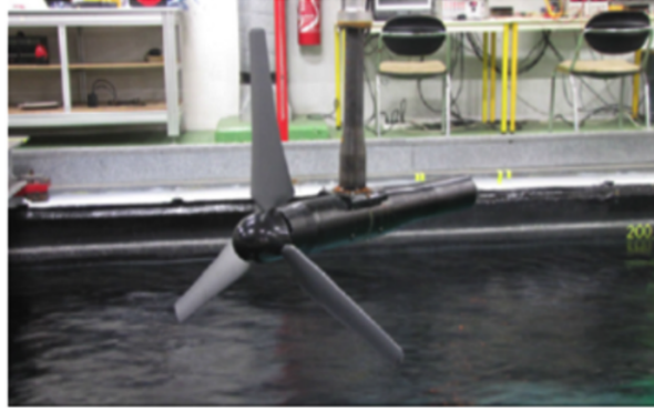
Fig. 3.7: Experimental turbine used in the IFREMER experiments (Mycek et al., 2014).
