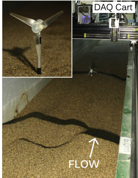
Fig. 1.16: Photo of single turbine with bedforms during experiments of Hill et al. (2015).
