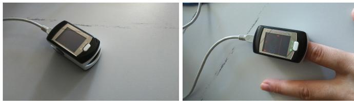
FIGURE 3.4 – The contact PPG sensor.
