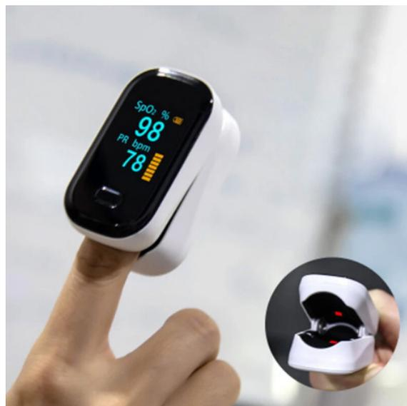
FIGURE 1.6 – Pulse oximeter (source : BOXYM oFit2 FingerClamp Pulse Oximeter).
