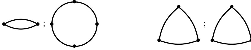
FIGURE 2.3: Two possible decompositions of the diagram of Fig. 2.2b into simple cycles.
