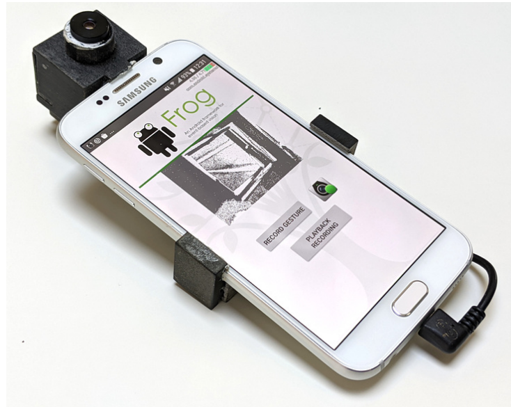
Fig. 3.2 Prototype device, consisting of a Samsung Galaxy S6 and a small form-factor ATIS connected via mini-USB port. The camera is held in place with a 3D-printed frame that attaches to the phone.
