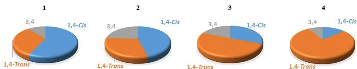
Figure 2.3. Microstructure content of the polyisoprene obtained from 1–4 /MAO catalytic systems
