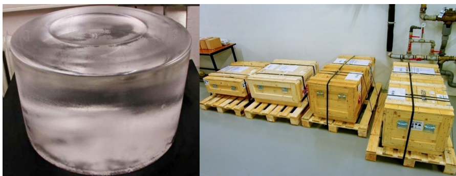
Figure 15: Photo of a IM substrate after the final forming step at Heraeus (left), so before any saw cutting. Example of shipment boxes for the substrates (right), ready for world-wide expedition. Photo credit : Heraeus and Laurent Pinard.
