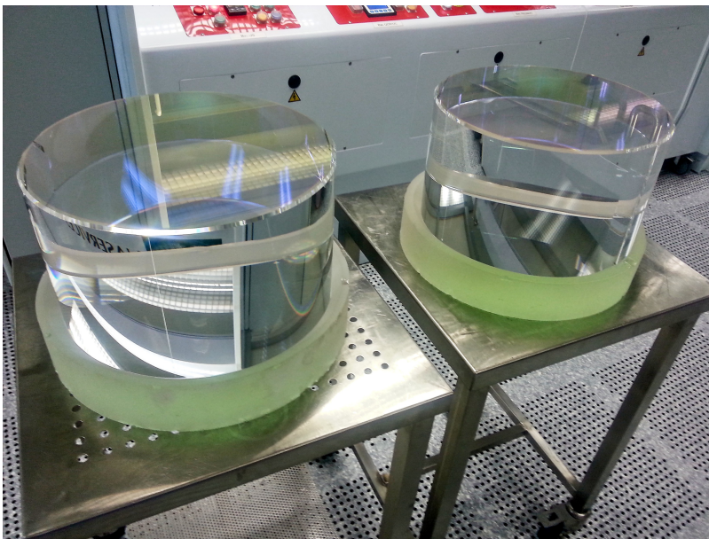
Figure 4: Photo of two arm cavity mirrors. They are cylindrical mirrors with a diameter of 350 mm for a thickness of 200 mm. Each one weights around 40 kg. Photo: L. Pinard
