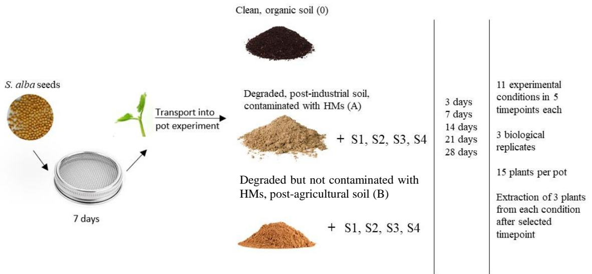
Figure 1. Experiment design. [0 – organic, peat soil, A – soil contaminated with HM by industrial activities; B – degraded but uncontaminated, post-agricultural soil; S1 – municipal sewage sludge contaminated by HMs; S2 – uncontaminated, municipal sewage sludge; S3 – industrial sewage sludge after purification of mineral water and beverages, S4 - industrial sewage sludge after purification of drinking water with high iron content].
