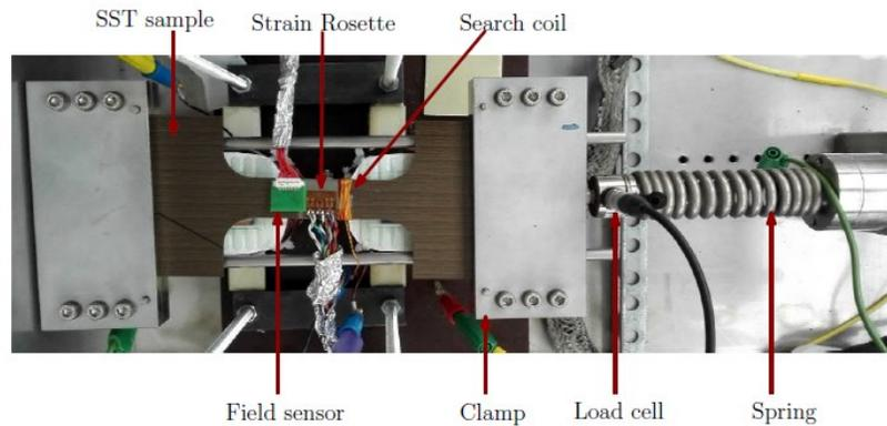
Fig. I.31 SST characterization device under uniaxial stress [46]
