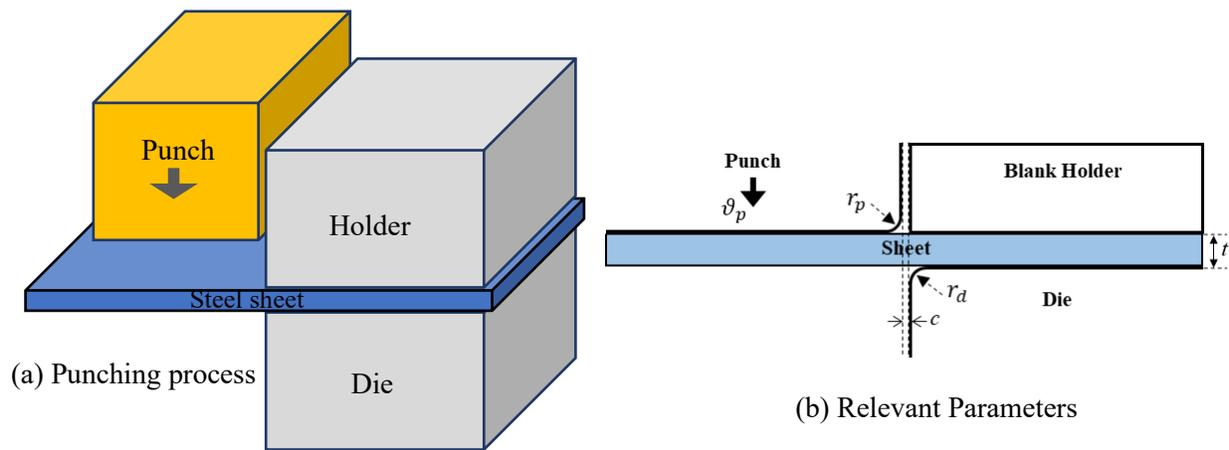
Fig. III.6 Schematic illustration of a conventional punching process
