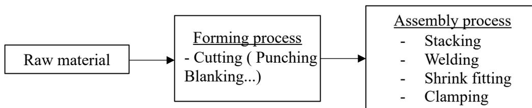
Fig I.13 Manufacturing processes of an electrical machine
