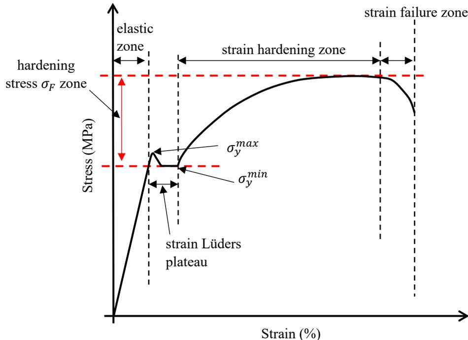
Fig. I.19 Stress strain curve of an electrical steel
