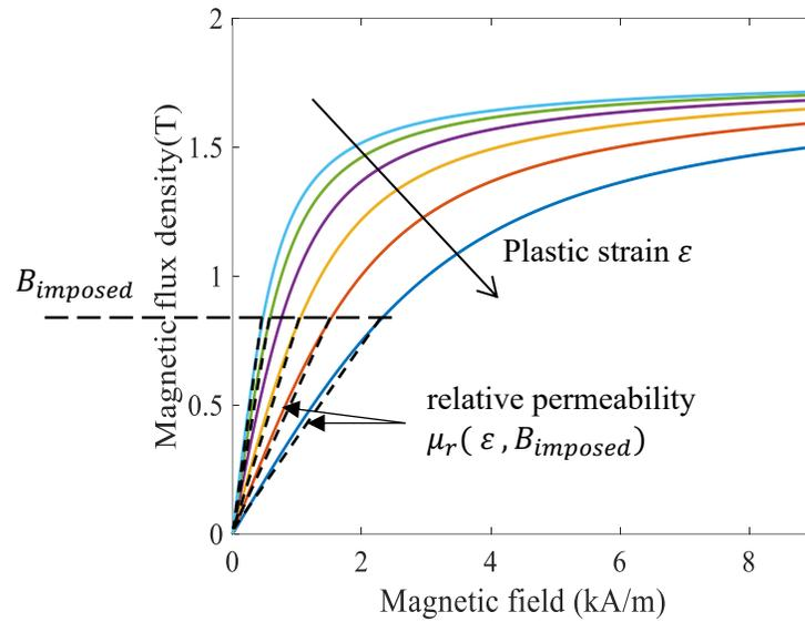
Fig. IV.26 Calculation method of the weighted degradation  $\omega_{i,j}$
