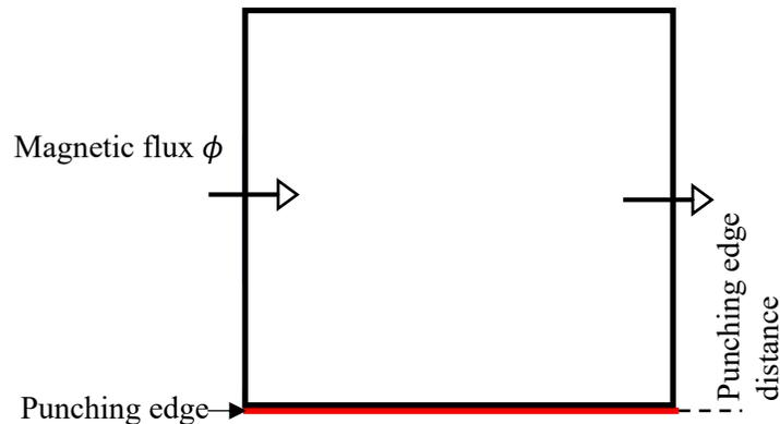
Fig. III.18 2D magnetostatic problem – a punched steel sheet
