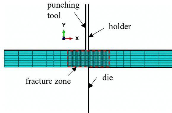
Fig. III.9 Schematic of the 2D simulated problem
