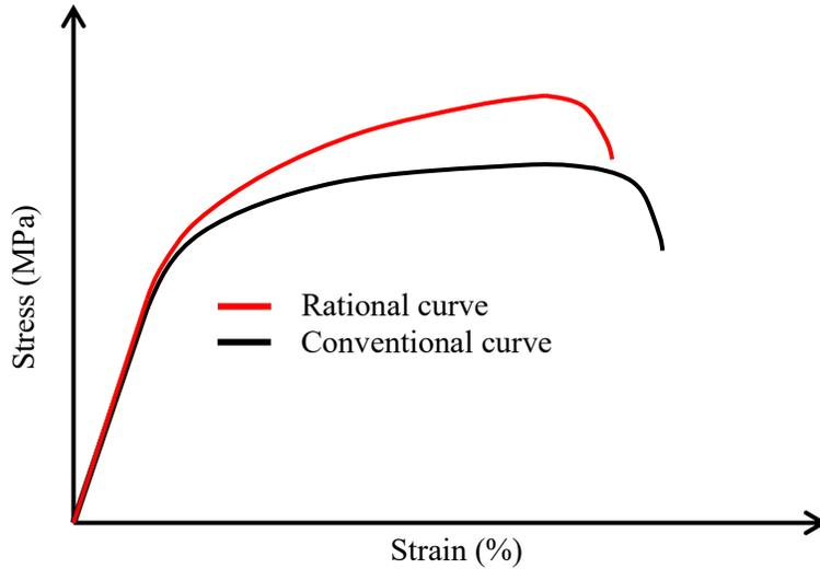
Fig I.11 Stress-Strain behavior: conventional curve and rational curve
