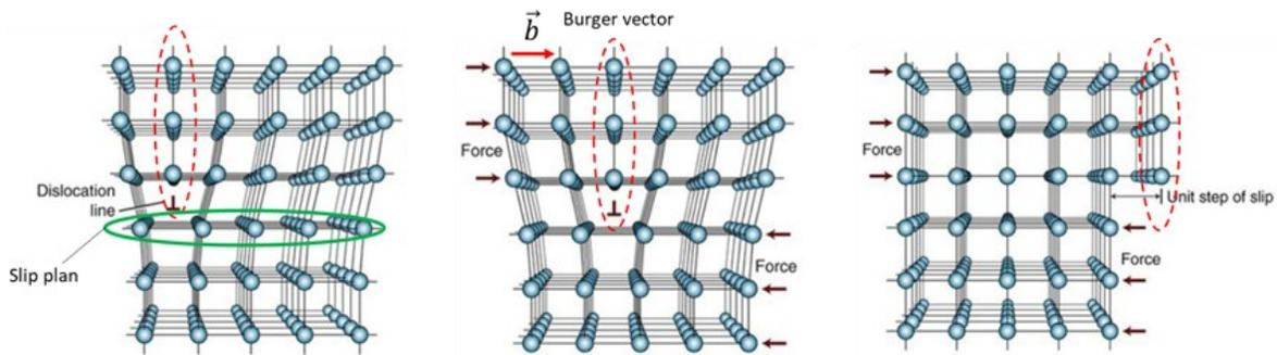
Fig. I.7 Mechanism of generation and motion of edge dislocation [8]
