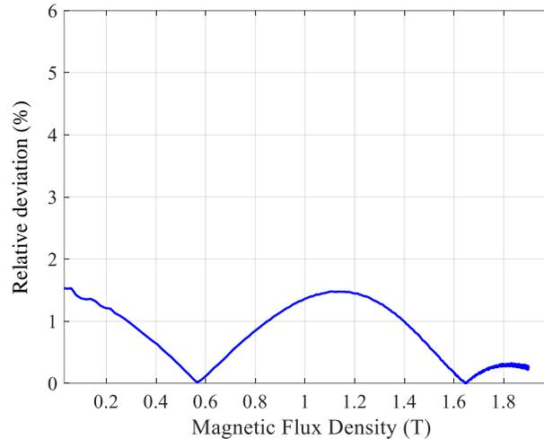
Fig III.5 Relative deviation of the Padé approximation method
