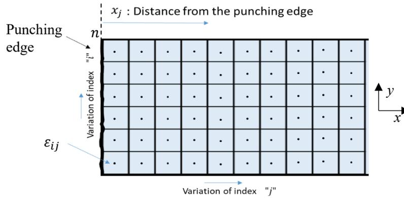
Fig III.14 Calculation method of the degradation profile
