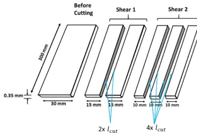
Fig. I.16 Schematic of the cut samples [18]
