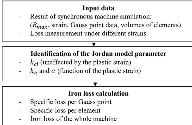
Fig. IV.9 Steps of the iron loss calculation
