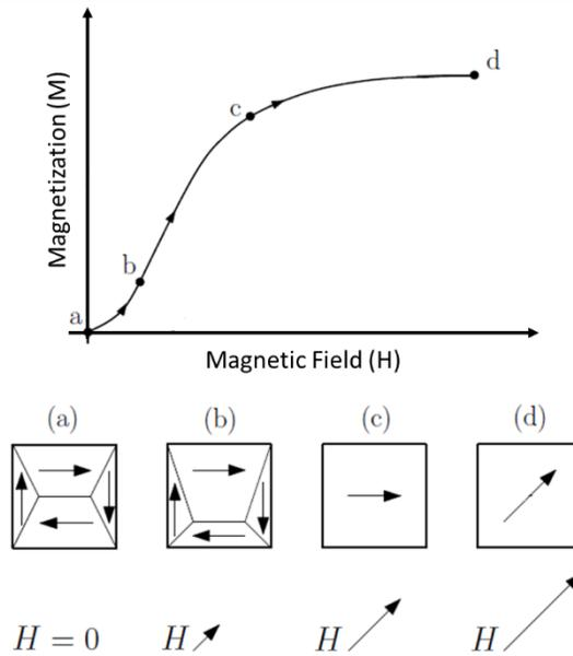
Fig I.4 Mechanism of ferromagnetic material magnetization [6]
