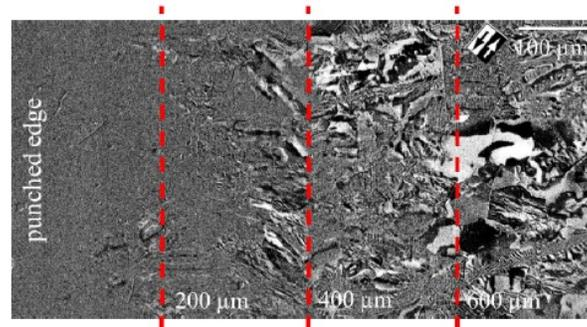
Fig. I.15 Typical MOKE micrograph near a cutting edge [15]
