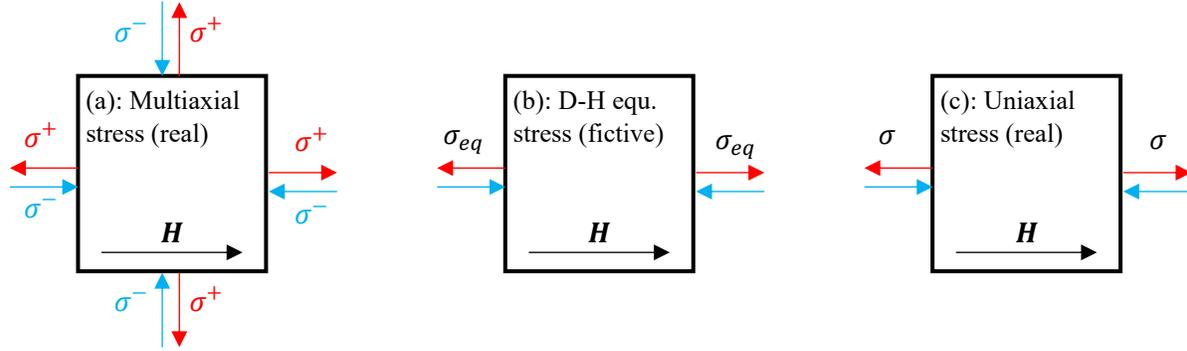
Fig. II.4 Illustration of bi-axial and equivalent stress configurations
