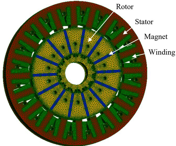
Fig. IV.6 Description of the simulated synchronous machine
