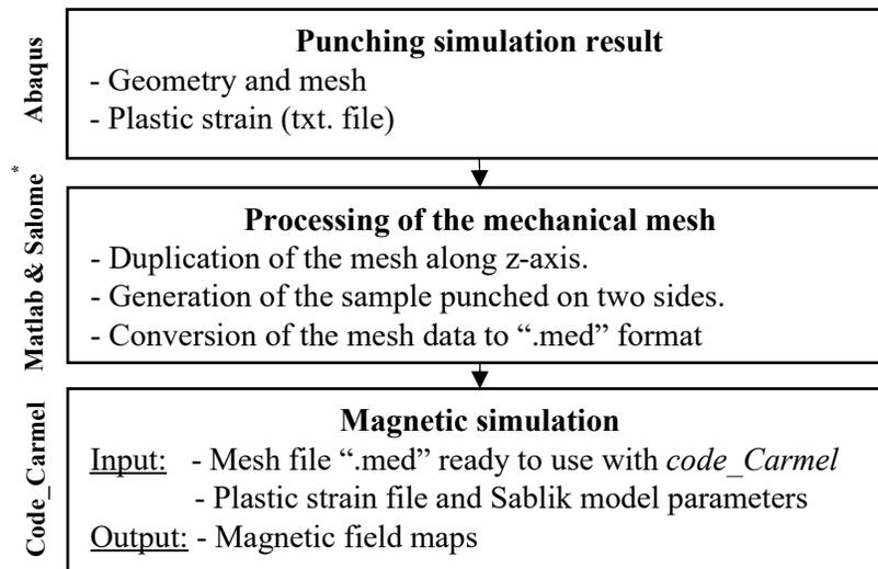
Figure IV.12 Principal steps of the mesh transformation operation.
