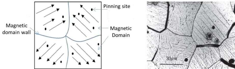
Fig. I.2 Domains in a polycrystalline sample 3% Si-Fe [5]
