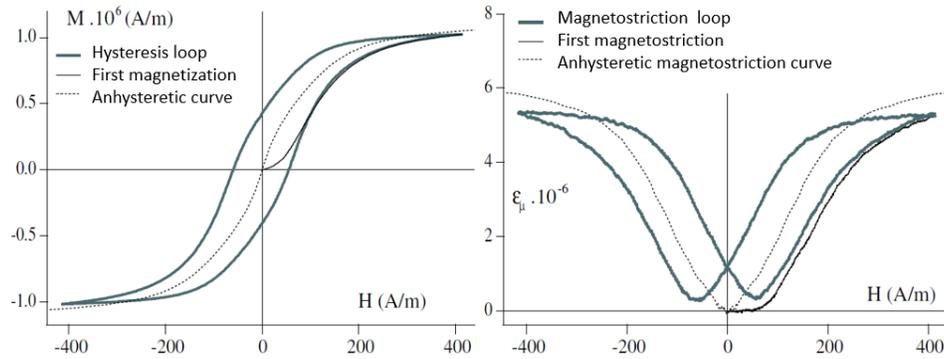
Fig I.26 (a) Magnetic behavior (b) Magnetostrictive behavior [44]
