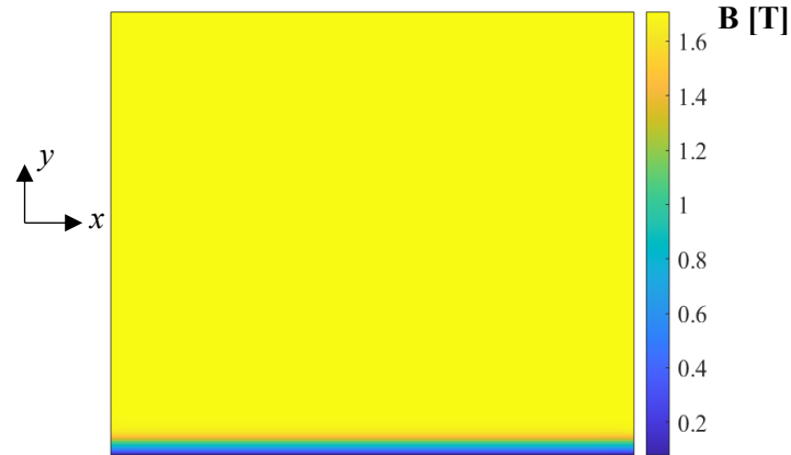
Fig. III.20 Distribution of the magnetic flux density in a steel sheet sample 3 \times 3 \text{ cm}^2 punched at the bottom with an imposed magnetic flux \phi = 0.05 \text{ Wb} .
