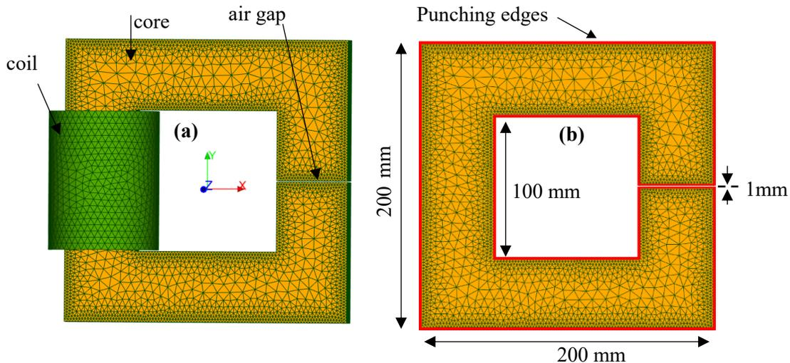
Fig. IV.1 Mesh and dimensions of the magnetic core
