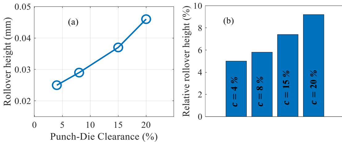
Fig. III.12 (a) Evolution of the rollover height versus punch-die clearance (b) relative rollover height
