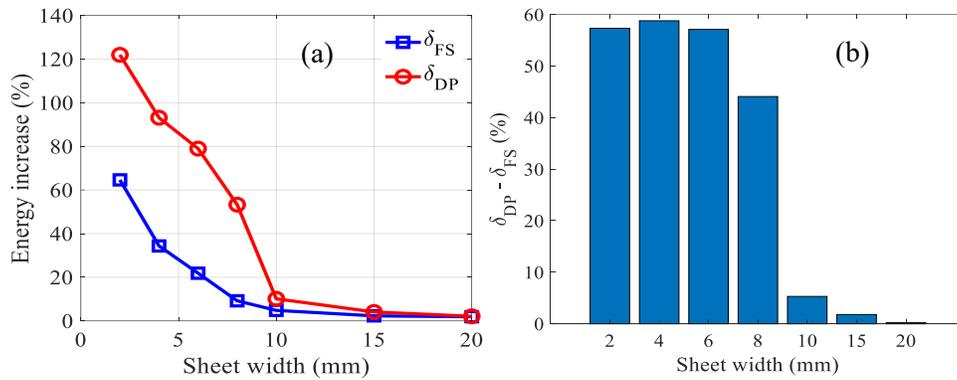
Fig. IV.20 (a) Evolution of the magnetic energy increase due to the punching effect for different sheet widths punched on two sides. (b) Difference in increase of magnetic energy  $\delta_{DP} - \delta_{FS}$
