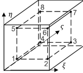
Fig. III.3 Location of the Gauss points in a reference hexahedron element [102]
