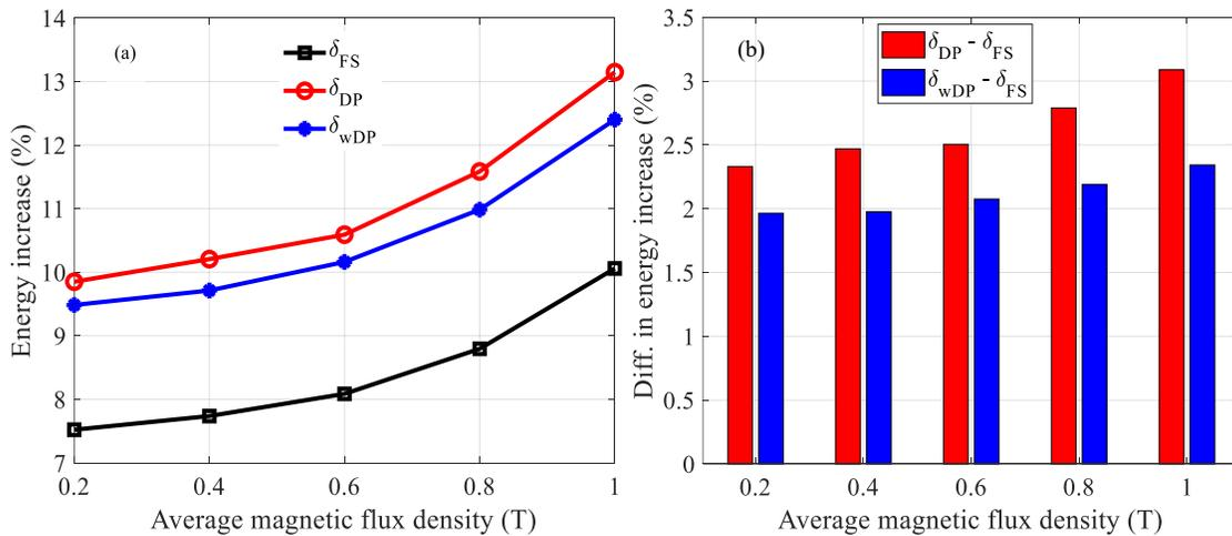
Fig. IV.28 (a) Evolution of  $\delta_{FS}$ ,  $\delta_{DP}$  and  $\delta_{wDP}$  for different imposed magnetic flux densities (b) difference in energy increase:  $\delta_{DP} - \delta_{FS}$  and  $\delta_{wDP} - \delta_{FS}$
