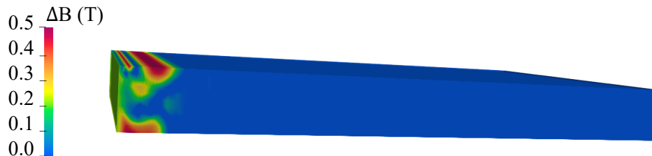
Fig. IV.15 Difference between magnetic flux density distribution obtained with the full plastic strain distribution and the degradation profile.
