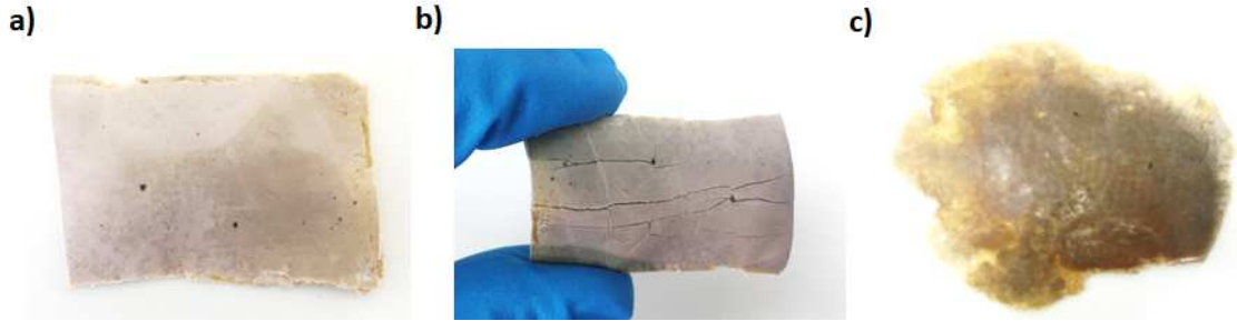
Figure ESI 16. Mechanical recycling of ELO/DTBA with 5wt.% PLA: virgin (a), damaged (b), repaired (c)
