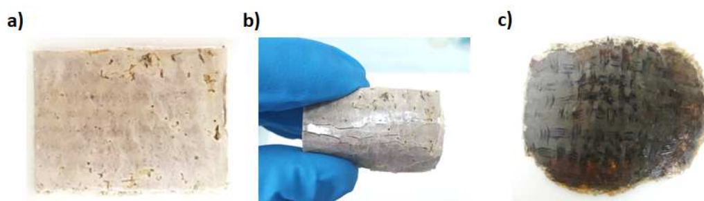
Figure 4. Mechanical recycling of ELO/DTBA/20% FF: virgin (a), damaged (b), repaired (c)
