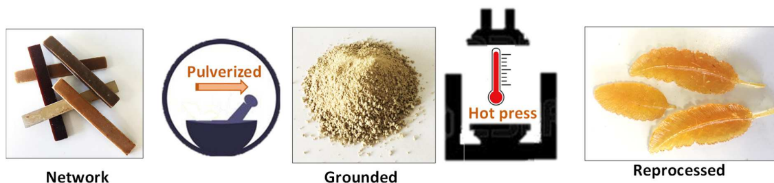
Figure 2. Mechanical reprocessing of ESFO/DTBA thermoset by hot pressing
