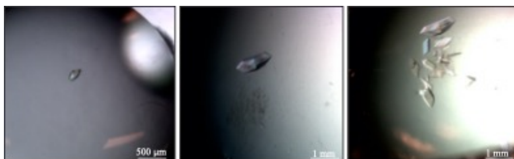
Figure 16. Growth of D-TIM E97Q crystal macro seeded into a sitting drop vapor diffusion experiment. A sitting drop with 1:1 ratio of 10 mg/ml D-TIM E97Q complex with 2PG and reservoir solution (12 % w/v PEG 2000) was prepared and sealed before fishing seed crystal. The seed crystal was taken from another sitting-drop vapor diffusion experiment consisting 16% PEG 2000.
