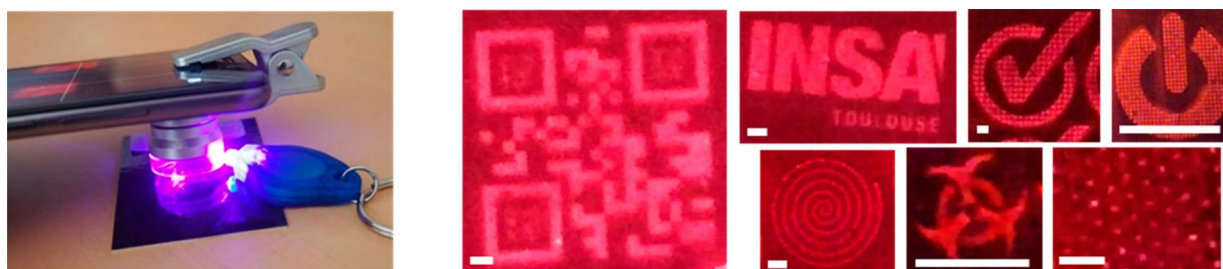
Figure 5. Reading of various PL tags using a smartphone equipped with a 20 \times clip lens. Scale bars are 100 \mu m.
